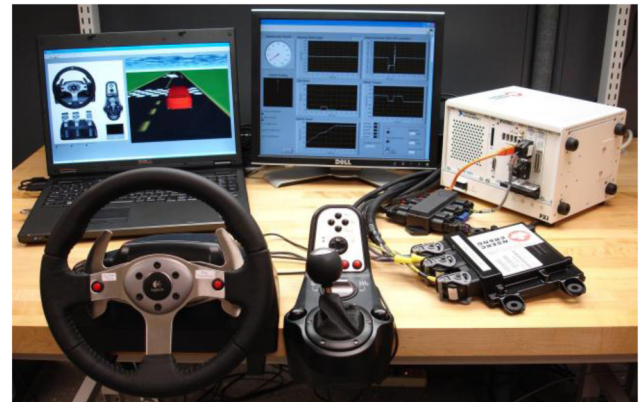
Figure 23. Hardware- and operator-in-the-loop driving simulator equipment
