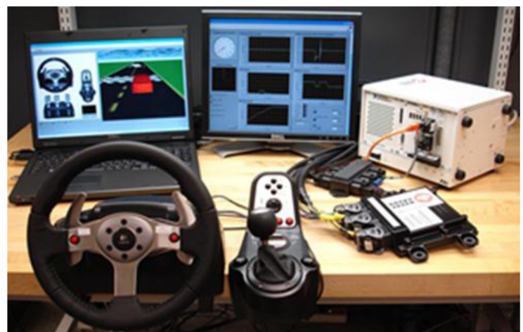
Figure 22. Hardware- and operator-in-the-loop driving simulator equipment
