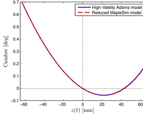
Fig. 2. Validation of camber for front SLEKQ model
