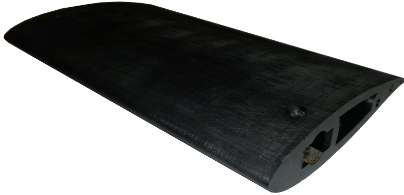
Figure 3.6: One of the five main 3D printed test blade sections
