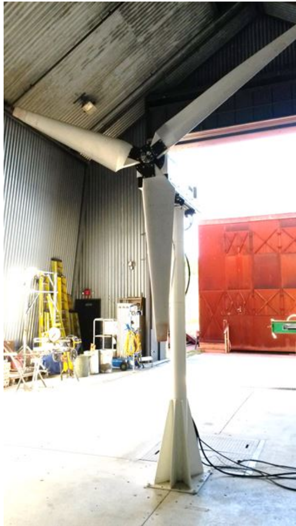
Figure 3.2: Photograph of the Wind Energy Group test turbine with Gertz [11] blades installed
