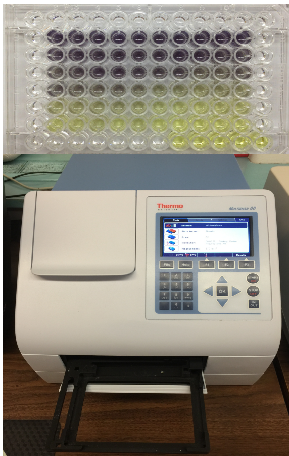
Figure 3-2: MTT assay performed in cells in a 96-well plate, and the plate reader.
