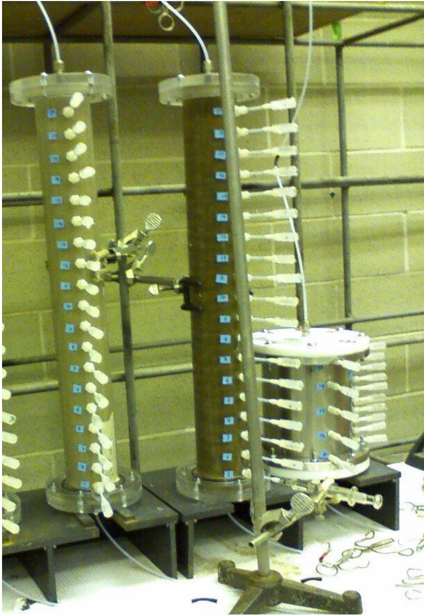
Figure 2-3 From left to right: Ottawa Sand Column (C2), Borden Sand Column (C3), and Borden Sand and GAC Column (C6); the picture shows the method of sampling using a glass syringe from port 1 of C3
