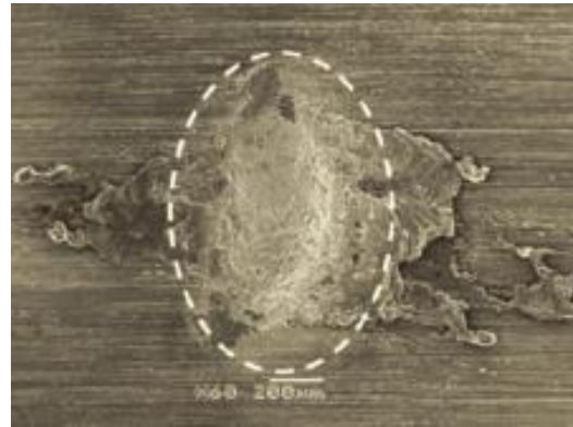
Figure 15: Surface of ESD crater using dynamic control mode [7]
