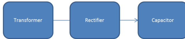
Figure 58: ESD Machine #1 electrical components block diagram [36]
