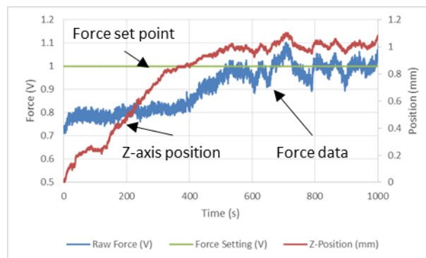
Figure 118: PID Controlled Force Test
