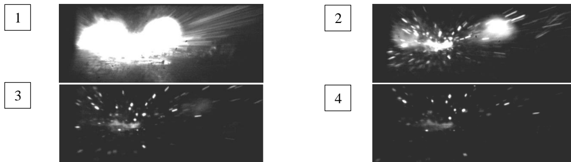
Figure 94 Test 3 135V, 300 \mu F and charging speed 95; 0.1ms per frame using a localized nozzle of 30CFH argon shielding gas
