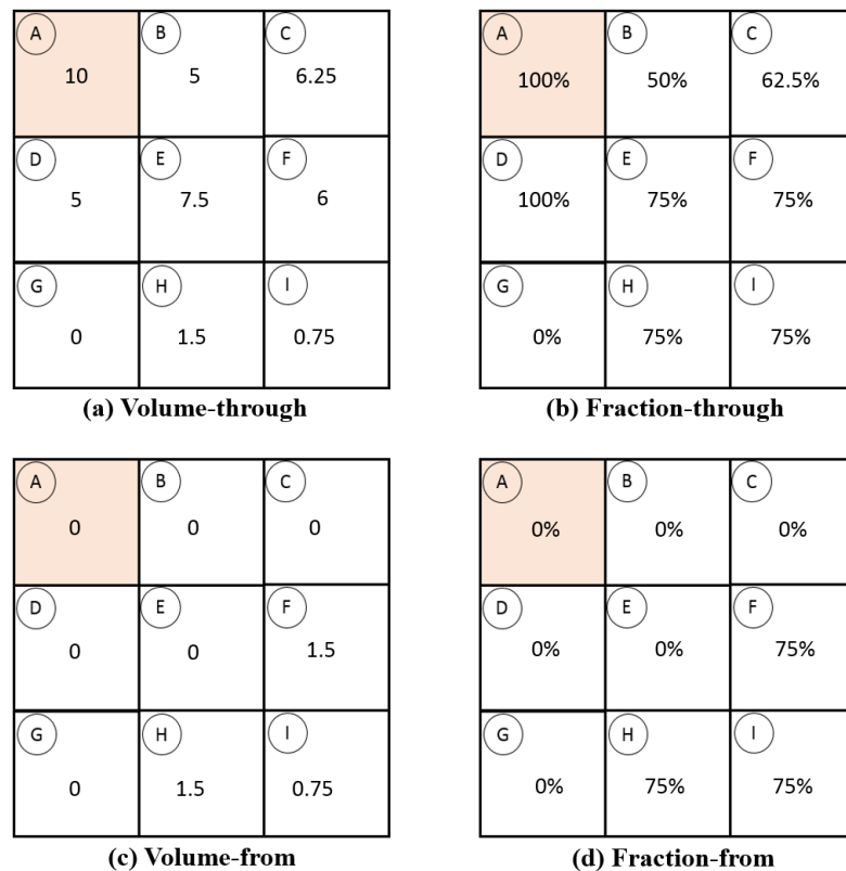
Figure 2.7. Calculated FlowSource metrics for the cell-by-cell flows from the example in Figure 2.4 (modified from Foley and Black, 2013).
