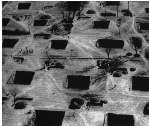
fig. 3.8 Cave dwellings in voids cut into the Loess Plateau in Northern Shaanxi Province
