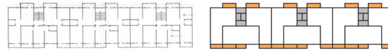
fig. 4.81 Plan of Socialist Era danwei housing with enclosed loggia and shared circulation stairs
