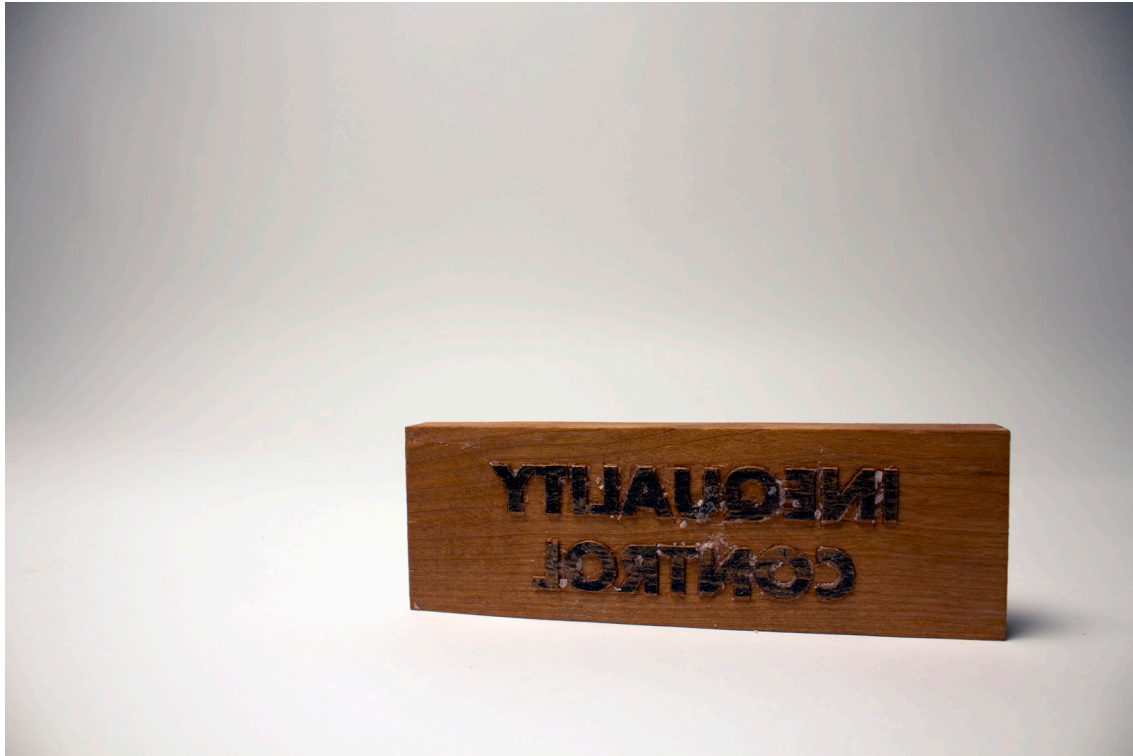
fig. 3.19. Second attempt at hand carved brick face for wax positive - black cherry
