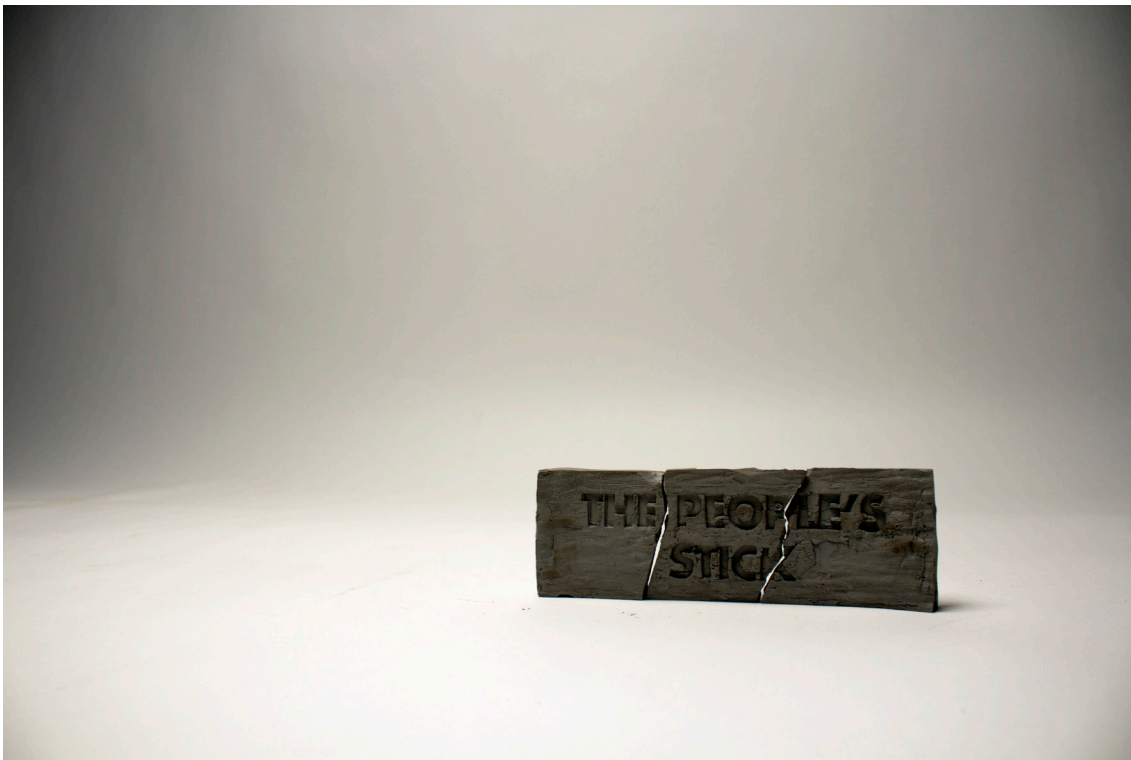
fig. 3.12. First attempt at slip cast brick - earthen slip
