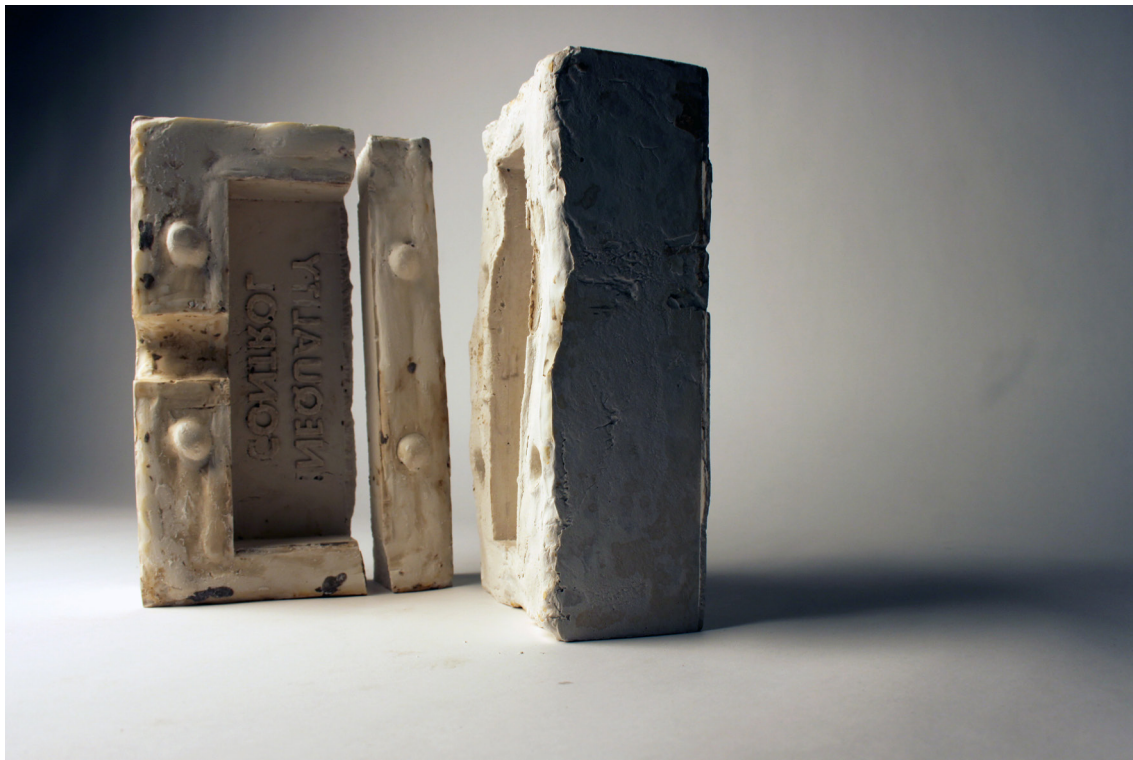
fig. 3.16. Resulting plaster cast from hand carved positive - hydrocal plaster
