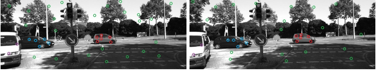
Figure 2.9: Example of motion segmentation by tracking point trajectories (shown by the circles). The different motion clusters labelled by colour, with green circles representing the background. Images obtained from KITTI autonomous vehicle dataset [23].
