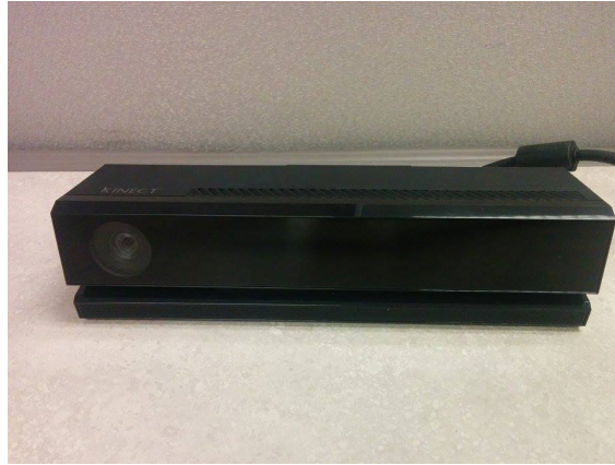
Figure 1.1: Example of an RGB-D camera. Shown above is the Microsoft Kinect v2 [53]
