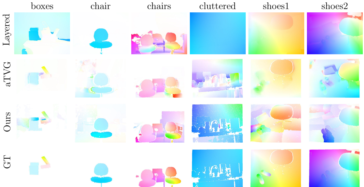
Figure 4.3: Visualizations of the estimated flow fields on the UW dataset. We can see that our method has difficulty matching homogeneous areas of the background motion, but can reliably estimate the flow of individual objects in the foreground. As expected, variational methods perform well to smooth out background motions.
