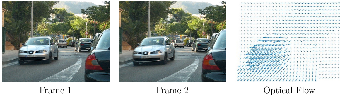
Figure 2.6: Optical flow example. Optical flow estimates the motion from frame 1 to frame 2, the downsampled 2D motion field is shown on the right. Images obtained from Human-assisted motion annotation dataset [48]
