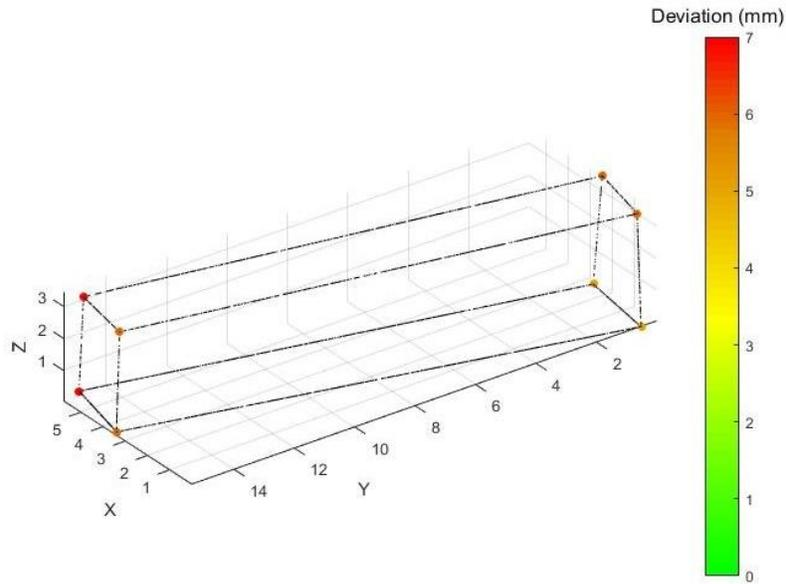
**Figure 56: Deviation analysis using MATLAB® code and surveying of eight key locations on the module in order to quantify dimensional variability associated with transportation loading.**
