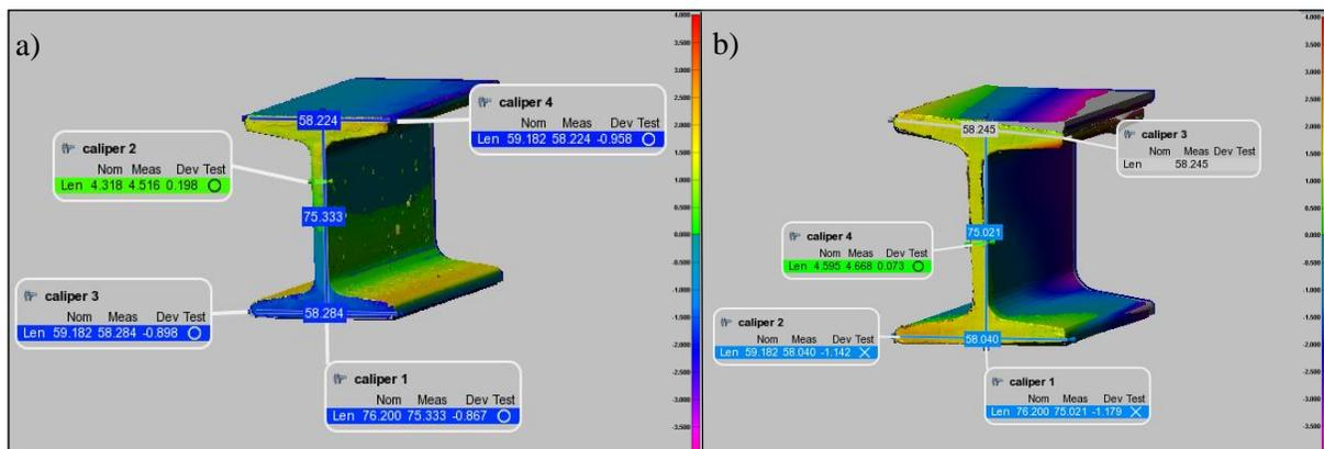
**Figure 18: PolyWorks® output for deviation analysis of S75x8 beam: (a) mill tolerances (b) geometric distortion (deviations shown are in mm)**
