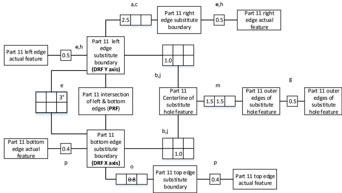
Part 11 (left) Diagram (inclined DRF from Part 9 DRF)
