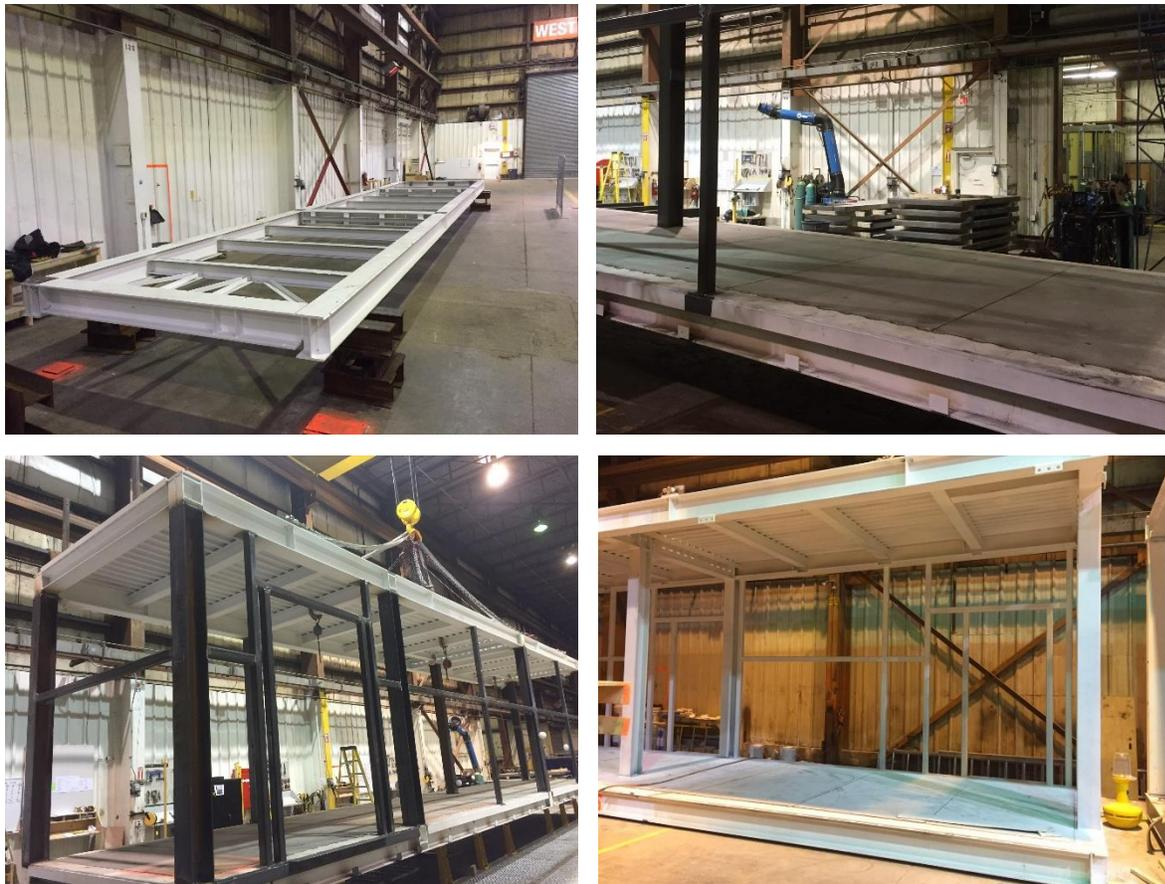
**Figure 40: Overall aggregation of the structural system. Top Left: floor frame. Top Right: concrete panels and columns installed on floor frame. Bottom Left: roof frame fit-up in place and installed on to columns. Bottom Right: completed assembly on shop floor.**
