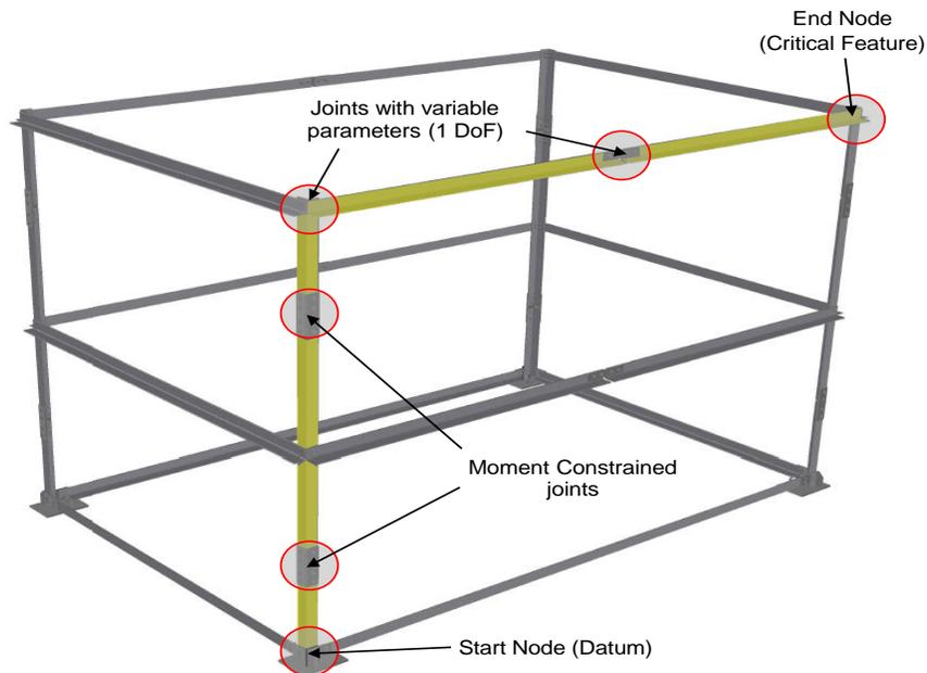
**Figure 63: A typical structural frame and a hypothetical assembly diagram (highlighted path). The joints with variable parameters are identified in the assembly path. The position of the critical feature is therefore modelled as a function of the joint parameters and variables.**
