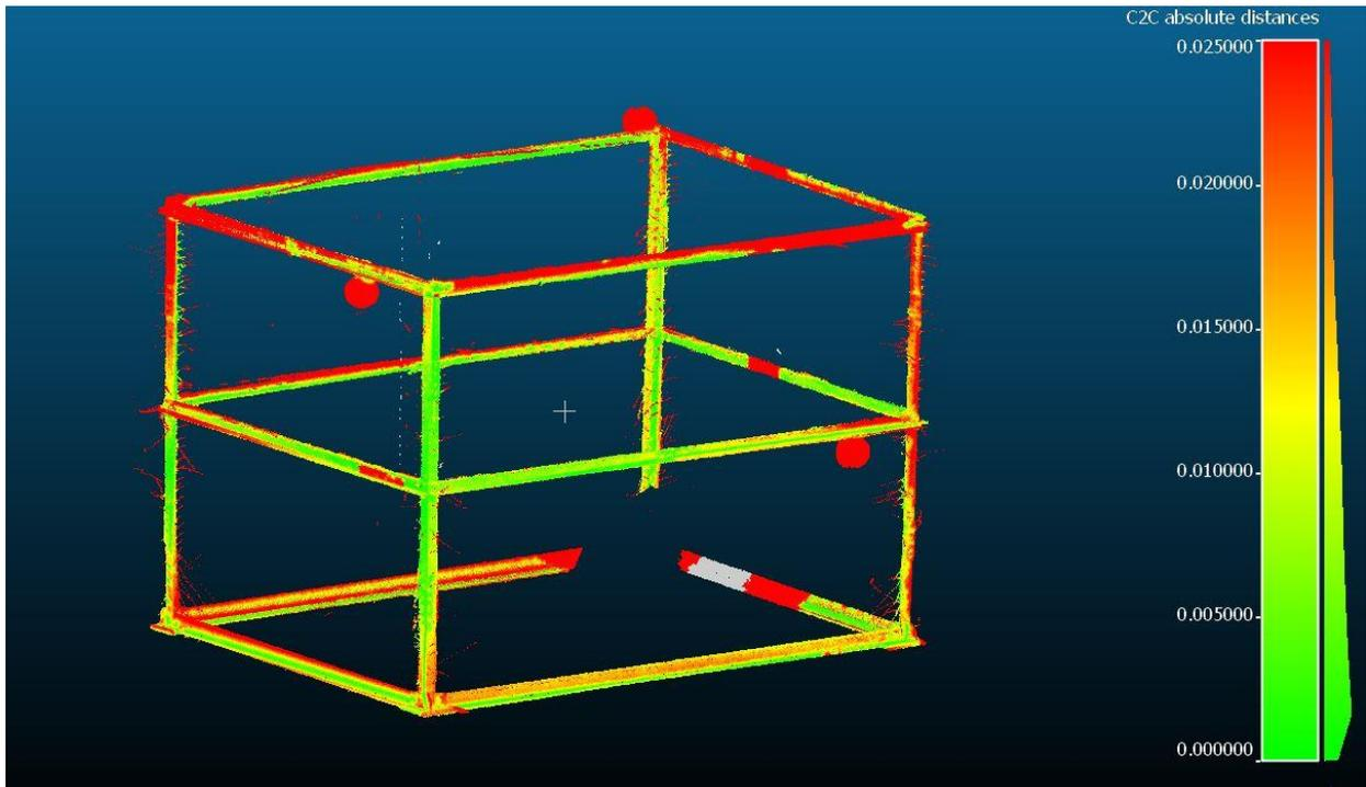
**Figure B5: Deviation analysis output for FARO® Laser Scanner 880 HE**
