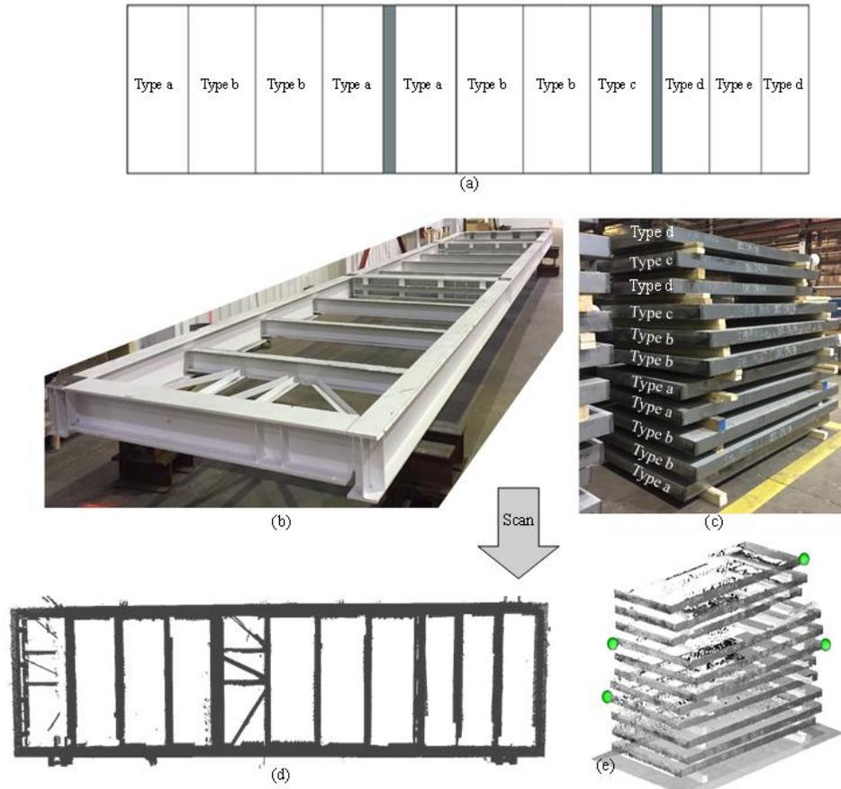
**Figure 91: Case II: full scale concrete panels. (a) Assembly plan and the panel types for each slot in the floor frame. Images of the floor frame (b), and the stack of the concrete panels (c). Laser scan of the floor frame (d), and the stack of concrete panels (e).**
