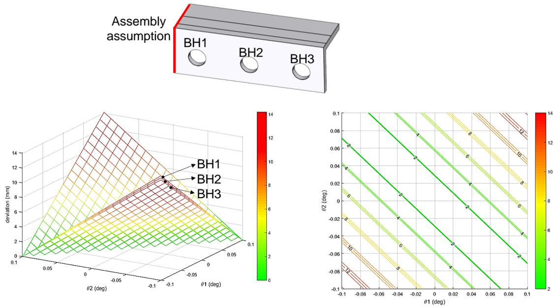
**Figure 70: Typical results for model-based DVA. Deviation surfaces and contour lines for the bolt holes (BH) are illustrated. The results are shown for the tie-in plate 2 (TP2) illustrated in Figure 68.**
