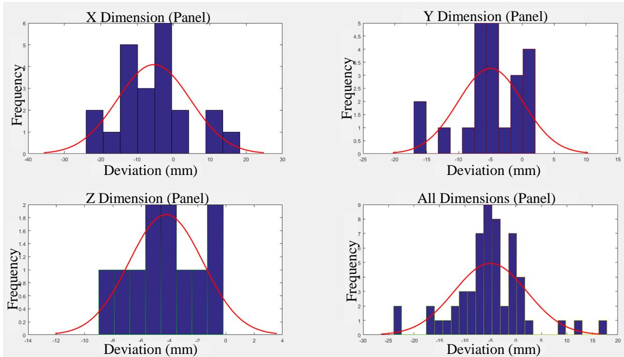
**Figure 28: Histogram plots for dimensional variability of concrete panel as-built dimensions.**
