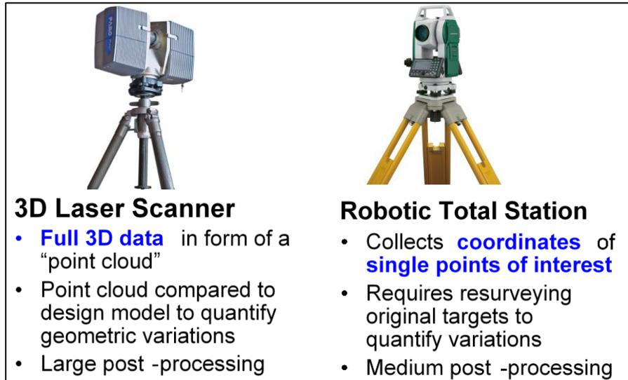
**Figure 23: Comparative overview of 3D laser scanning versus robotic total station for as-built data collection (FARO 2007, Sokkia 2015)**
