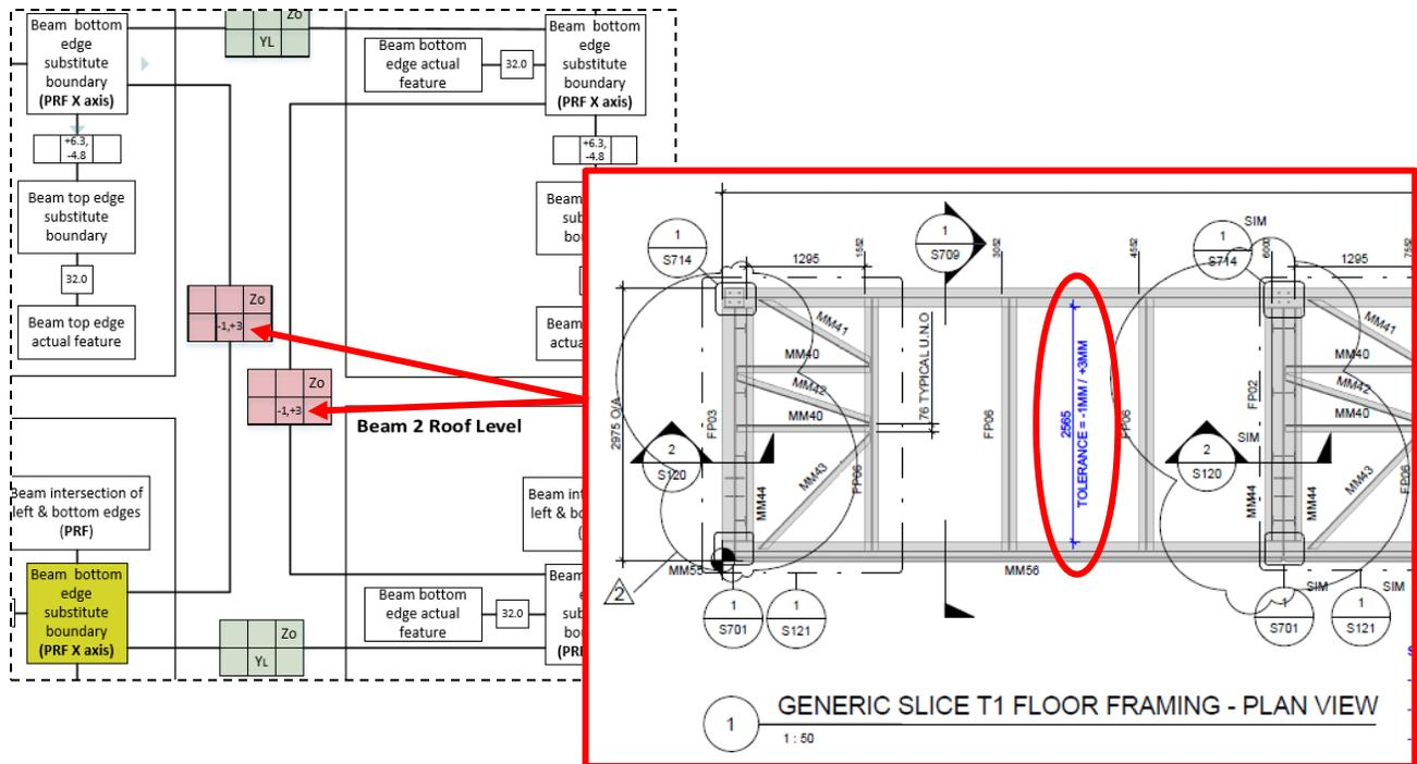
**Figure D33: Derivation of Positional Tolerances in Y-dimension between Beams in Case Study 2**
