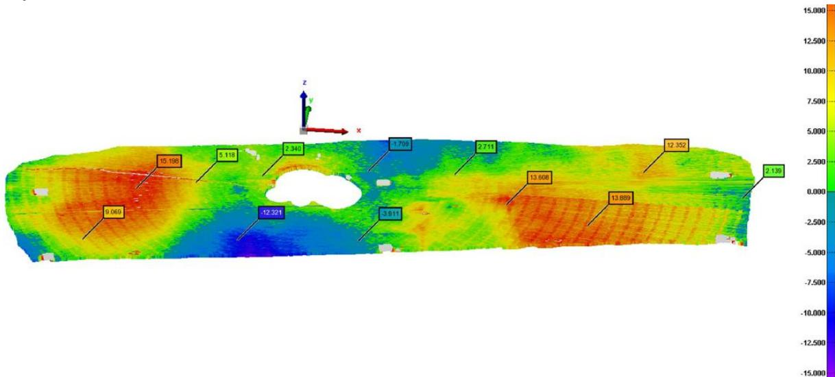
**Figure 48: Plane deviation analysis output using PolyWorks® to assess the dimensional variability associated with the shop floor.**
