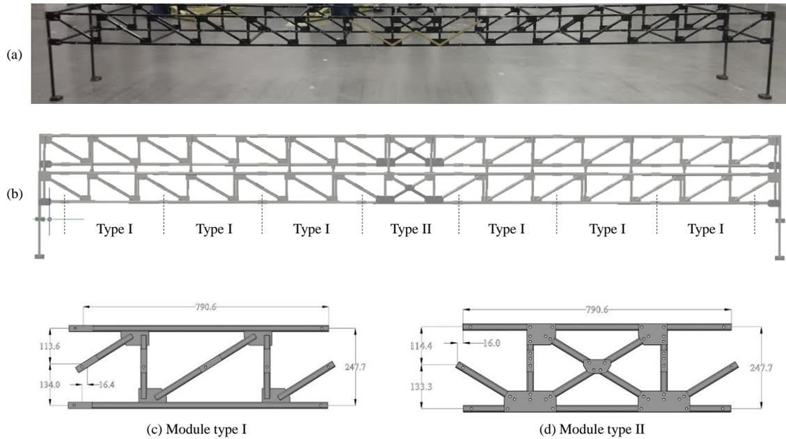
**Figure 87: Case Study I. (a) actual image, (b) 3D model the assembled bridge, dimensions of modules type I (c) and II (d). Dimensions are in mm.**
