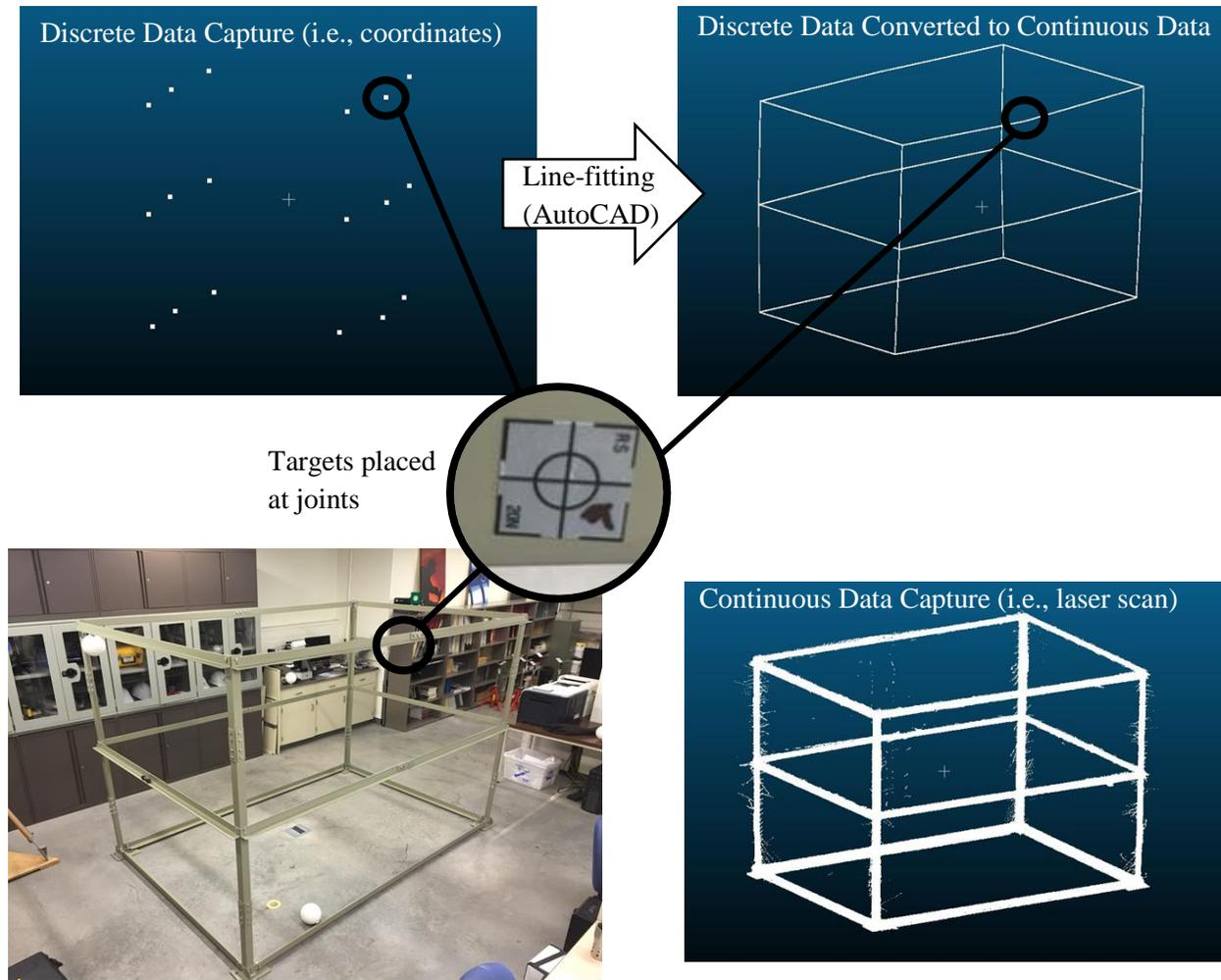
**Figure B3: Comparison of discrete data capture (i.e., total station and laser meter) versus continuous data capture (i.e., laser scanner)**
