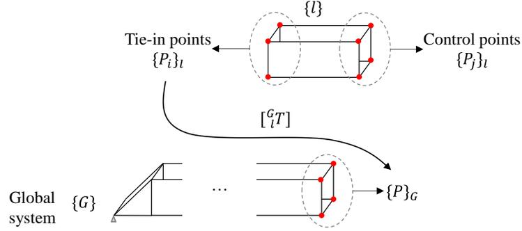
**Figure 83: Parameters for transformation of modular components from local to global coordinate system.**
