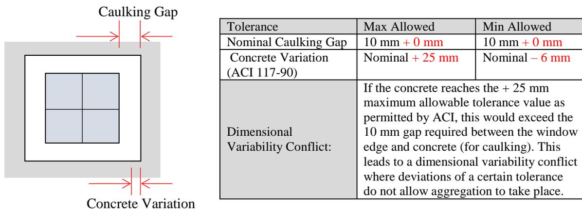
**Figure 6: Depiction of caulking gap and concrete variation (with explanation of tolerance values)**
