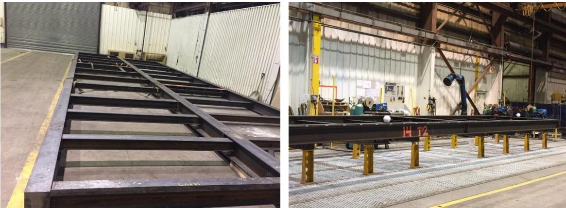
**Figure 30: Left: Standardized frame from outsourced supplier. Right: Standardized frame fit with custom bracing (note: custom bracing installed on framing table)**
