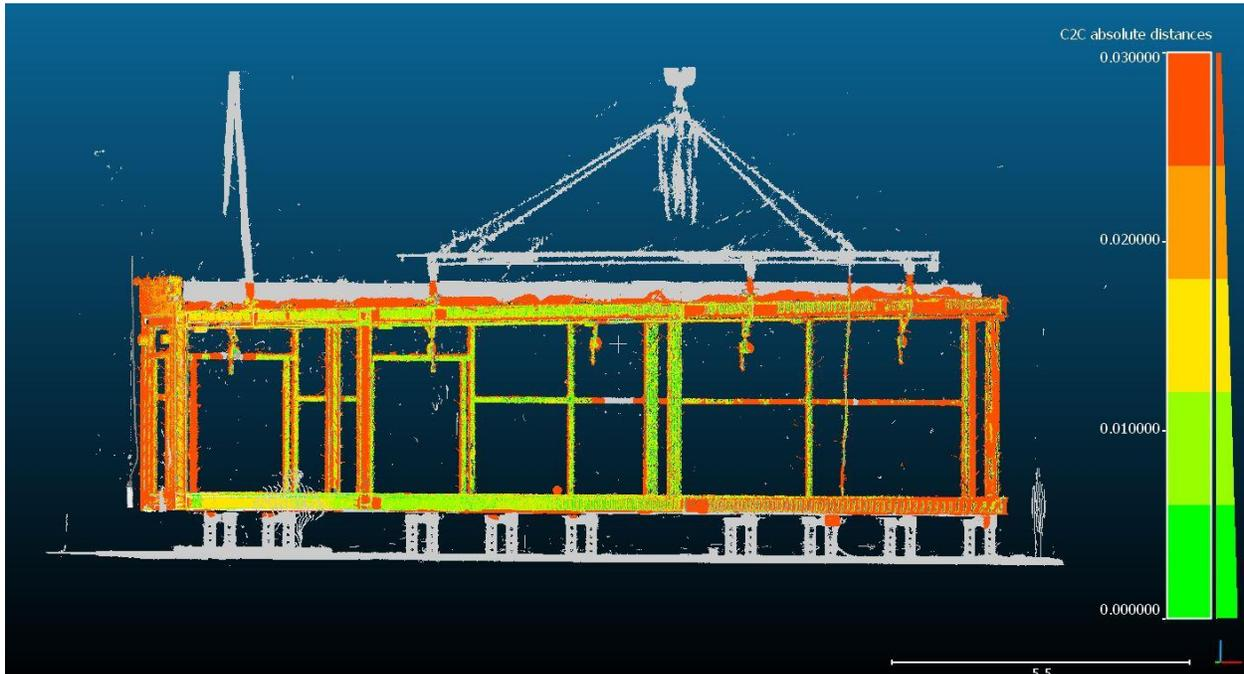
**Figure 53: Scan-to-scan deviation analysis using Cloud Compare® to quantify dimensional variability associated with geometric response of crane load (deviations shown are in m).**
