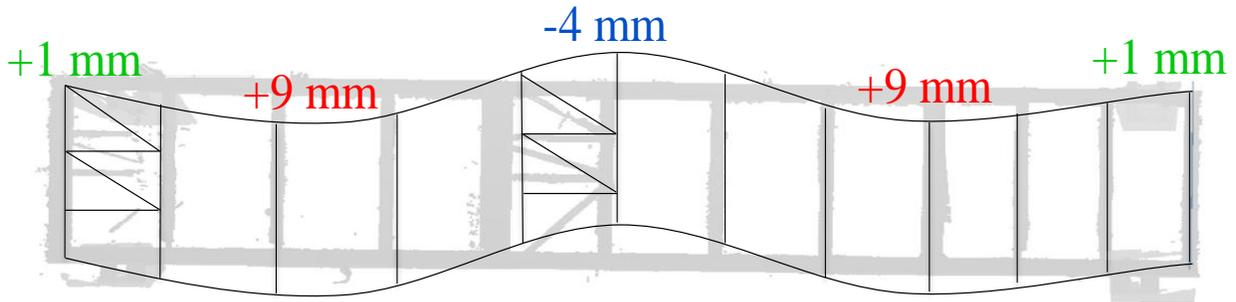
**Figure 35: Deviation pattern in the form of bowing along the lengths of a floor frame (not to scale)**
