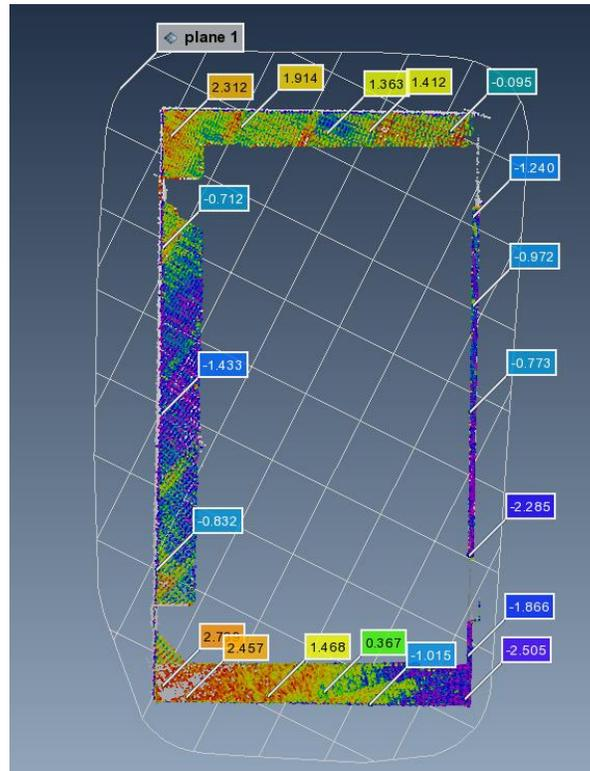
**Figure 29: Plane deviation analysis output using PolyWorks® of the top surface of a typical concrete panel (deviations shown are in mm).**
