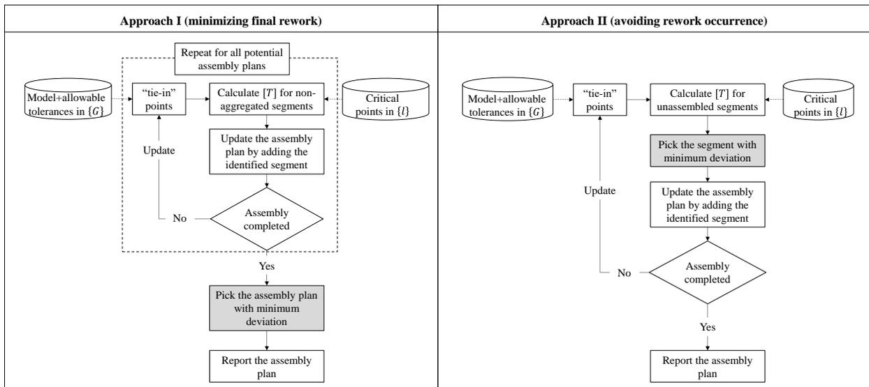
**Figure 84: Overview of the optimization strategies for assembly planning. Approach I: minimizing final rework, this approach finds all potential assembly plans and picks the plan with least resulting deviation. Approach II: avoiding rework occurrence, this approach minimizes the resulting deviation for each segment. Optimization steps for each framework are highlighted.**
