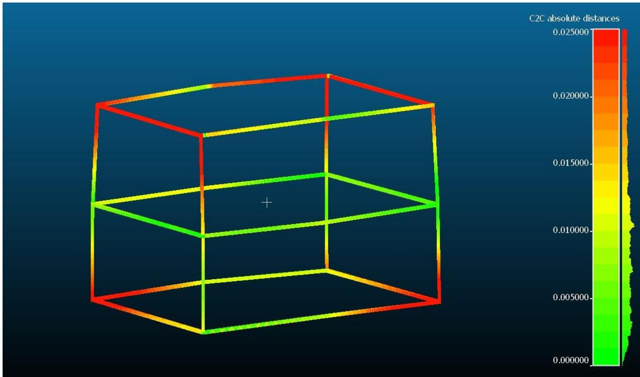
**Figure B6: Deviation analysis output for Sokkia® 30R Robotic Total Station**
