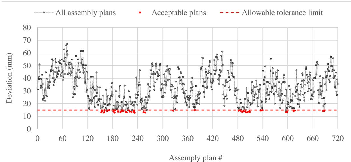
**Figure 90: The dimensional deviation for all feasible assembly plans for Case Study I. Number of possible assembly plans equals the permutation of 6 interchangeable modules ( $6! = 720$ ). The threshold value for acceptable deviation is considered 15 mm and all 51 assembly plans are identified as red points. The best five assembly plans are reported in Table 22.**
