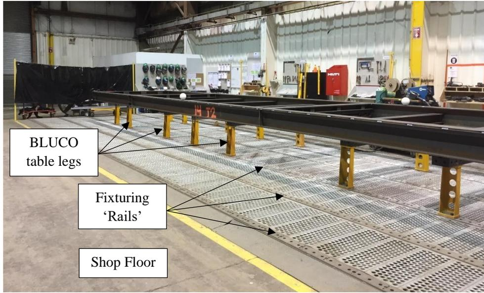
**Figure 46: Shop floor, BLUCO table legs and fixturing rails.**
