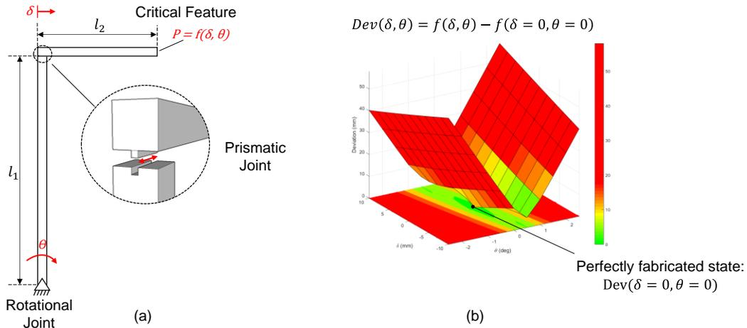
**Figure 66: Hypothetical example for dimensional variation analysis using kinematics chain. (a) An assembly with 2 DOF's, one rotational and one translational, is shown. (b) The position of the critical feature is therefore modelled as mathematical function of the two variables and constant links' length identifying the geometry. The critical feature's position function is shown as  $P = f(\theta, \delta)$ .**
