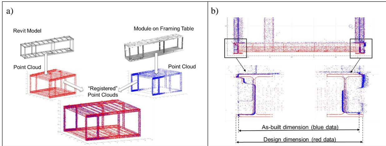
**Figure 19: Deviation analysis of commercial building module using: (a) registration of scan and BIM point clouds and (b) feature-to-feature comparison to quantify the dimensional quality of module width.**
