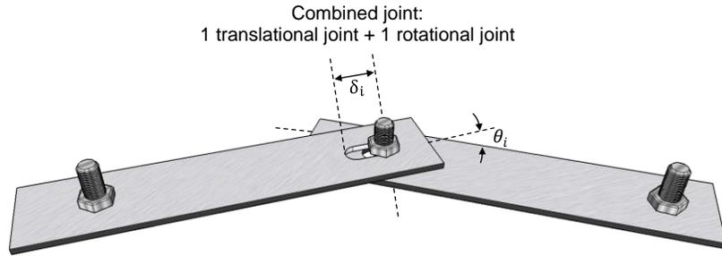
**Figure 65: Schematic of a hypothetical joint. The joint is combined of a translational joint and a rotational joint in parallel. The value  $\delta_i$  is variable for translational joints, and  $\theta_i$  is variable for rotational joints.**
