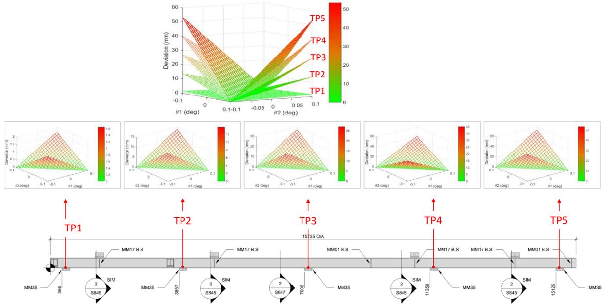
**Figure 73: Propagation of dimensional variation along the roof frame of the case study in different tie-in plates. As seen, tie-in plates further from the datum have higher impacts. Using kinematics chains and input from point cloud data yields output in the form of absolute deviations.**
