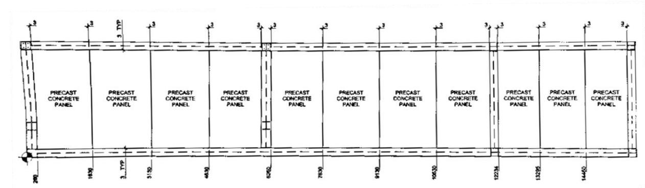
**Figure 26: Width of each precast concrete panel, with a 3 mm tolerance for spacing between panels**
