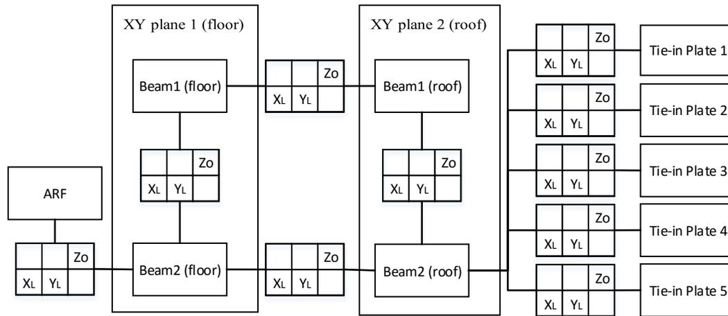
Figure D24: Assembly Diagram for Case Study 2 (Tie-in Plate Deviations)
