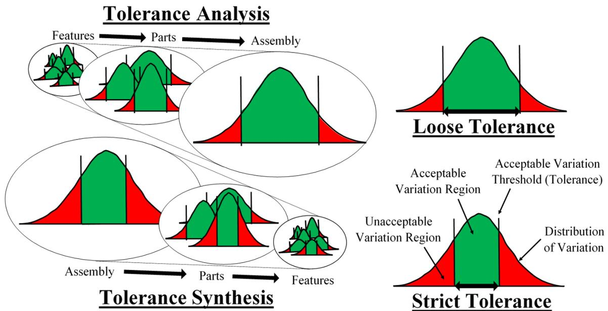
Figure A10: Sequence of specification for tolerance analysis and tolerance synthesis
