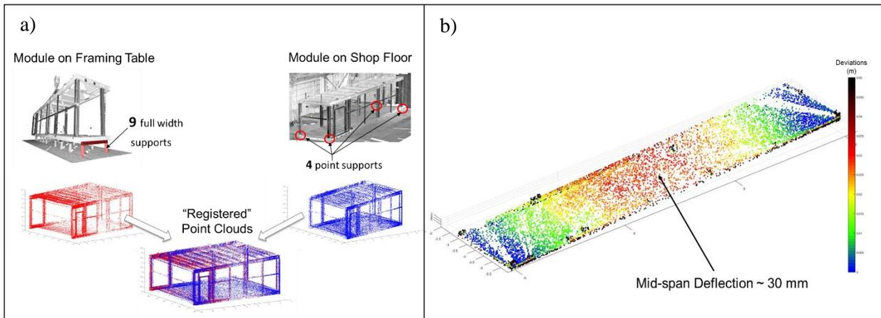
**Figure 20: Deviation analysis of commercial building module using: (a) scan-vs-scan registration and (b) point-to-point comparison to quantify deflection of module base while supported on shop-floor temporary cribbing.**
