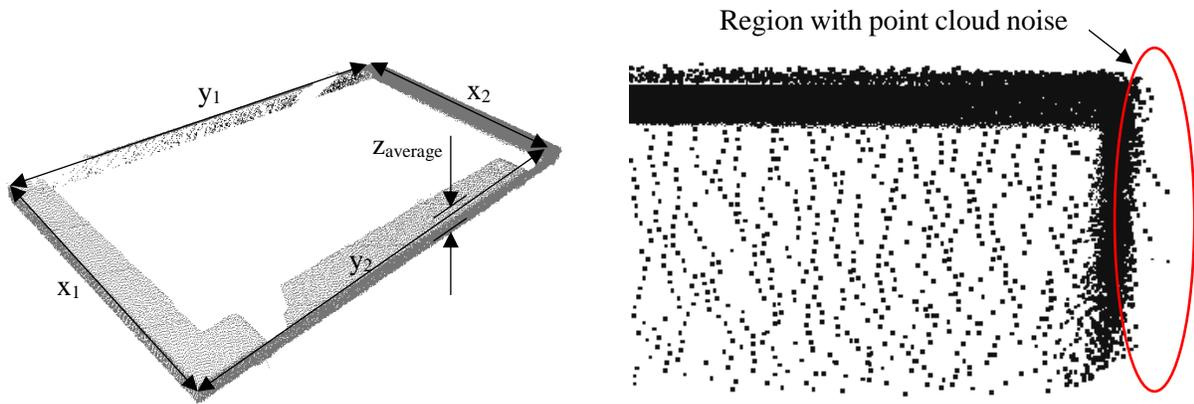
**Figure 27: Left: Sample point cloud with annotated dimensions extracted for each panel. Right: Sample point cloud with noise surrounding the perimeter of a precast concrete panel**
