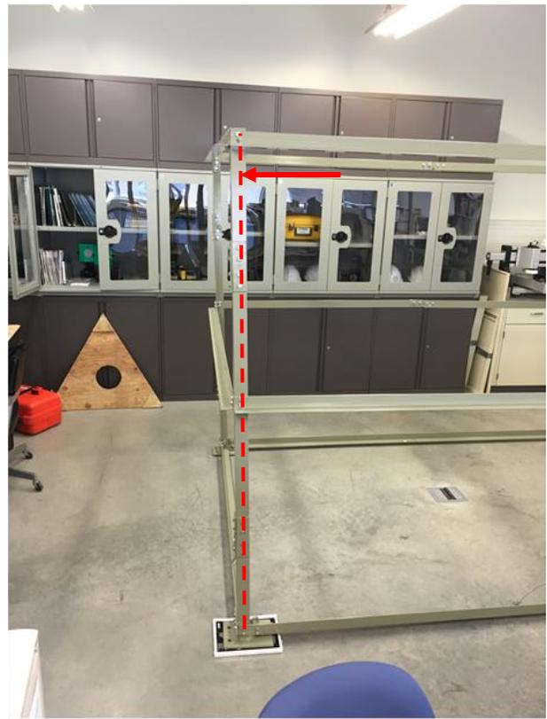
**Figure B2: Dimensional tolerance non-compliant state of test frame used for calibration (figure depicts sample misalignments along width and length at different joints)**
