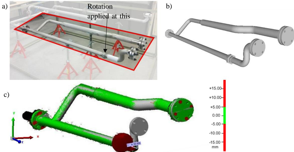
**Figure 21: Deviation analysis to compare: (a) the as-built state of pipe spool module, (b) to the BIM in order to quantify dimensional quality of module interface for alignment using (c) point-to-feature comparison**
