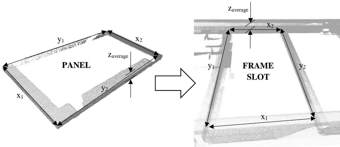
**Figure 31: Demonstrating critical dimensions from precast concrete panel (left) and the corresponding slot on the floor frame (right)**
