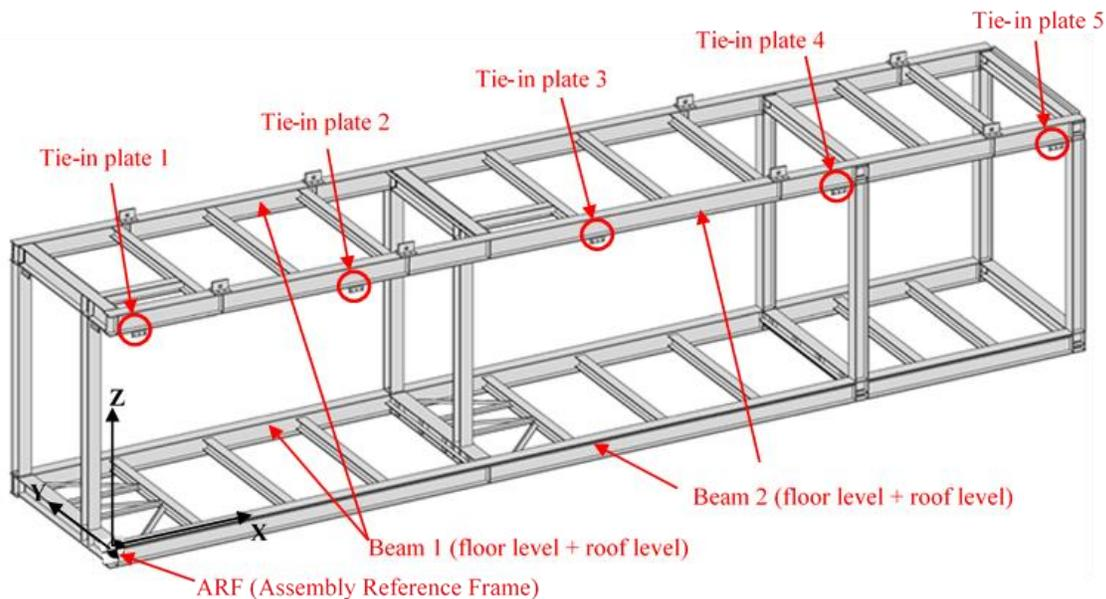
**Figure 60: 3D view of the module structure used in tolerance mapping case study 2 for outlining the position of tie-in plates along the length of the module with respect to the global datum (referred to as the Assembly Reference Frame).**
