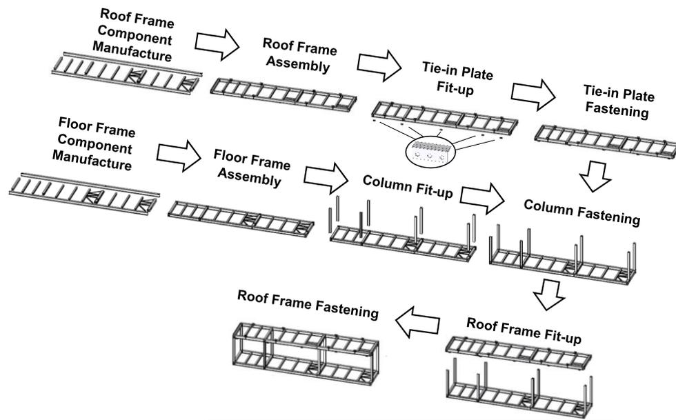
**Figure 24: Schematic representation of the key fabrication processes involved with construction of module structural system (with additional processes outlined for fit-up and fastening of tie-in plates).**
