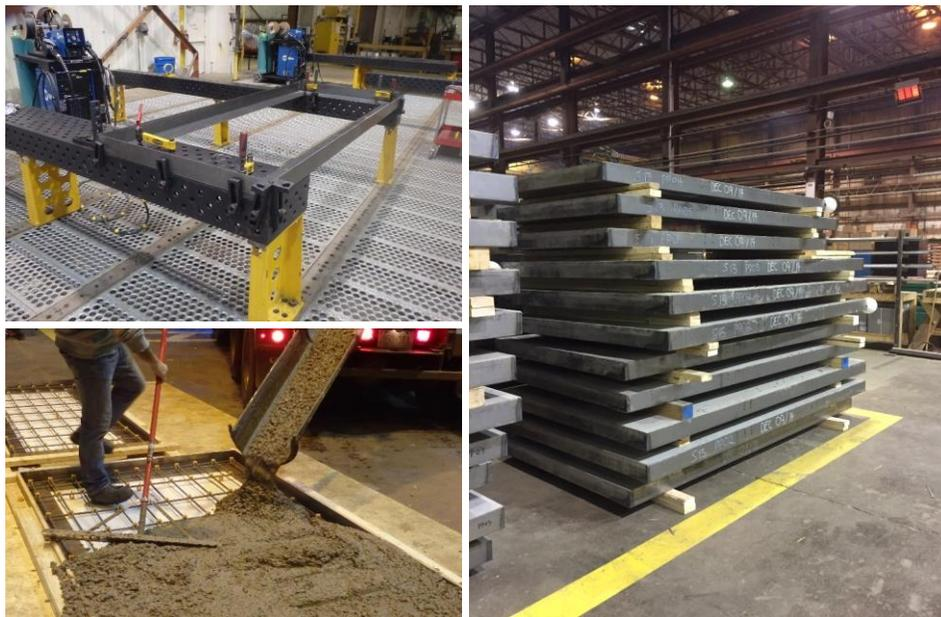
**Figure 25: Production of precast concrete panels. Top-left: fit-up of light-gage steel frame using framing table for dimensional control. Bottom-left: concrete pour. Right: concrete panels before aggregation in floor frame.**
