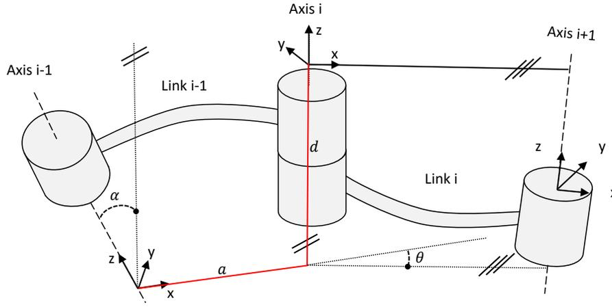
**Figure 64: Illustration of D-H parameters for a typical connection. D-H parameters are used for developing the kinematics chain to relate the geometric relationships of an assembly.**
