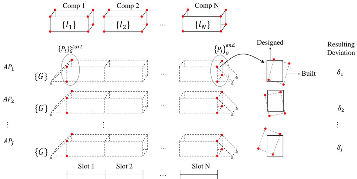
**Figure 85: Hypothetical example for optimizing the assembly plan using approach I (minimizing final rework). The assembly plan associated with the minimum  $\delta$  is picked as the plan that minimizes the dimensional deviation.  $\{l\}$  and  $\{G\}$  are local and global coordinate systems respectively.**
