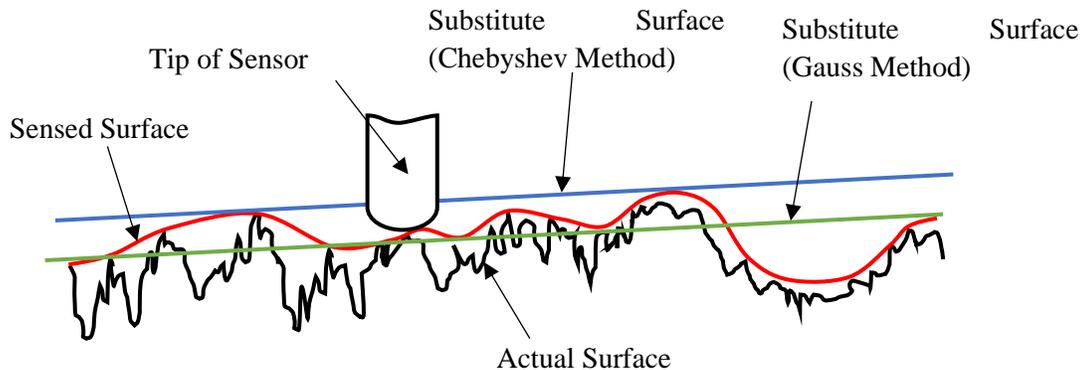
**Figure A7: Actual surface, sensed surface and substitute surface, adapted from (Miller et al. 1962)**
