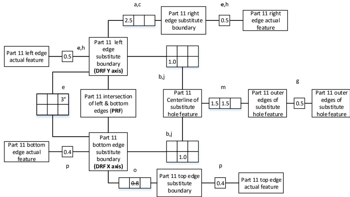
Part 11 (right) Diagram (inclined DRF from Part 9 DRF)
