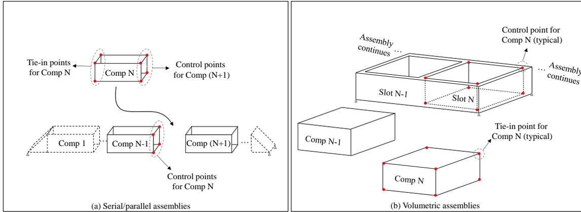
**Figure 81: Tie-in points and control points for: (a) serial/parallel assemblies, and (b) volumetric assemblies.**
