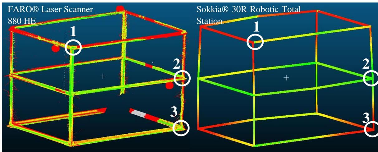
**Figure B11: Key differences between the critical joint coordinate data for discrete and continuous data capture devices**
