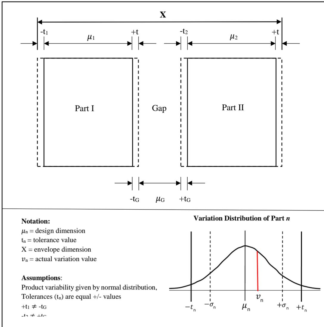
**Figure A5: Accumulating Dimensional Impact of Product Variability, Tolerances and Functional Gaps for Two Parts in an Assembly (Source: own)**
