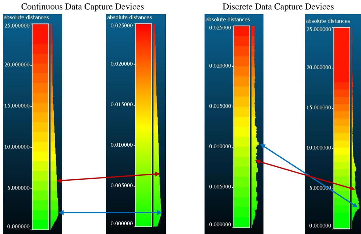
**Figure B10: Comparison of deviation histograms between data sets (left to right: Trimble® GX 3D Laser Scanner, FARO® Laser Scanner 880 HE, Sokkia® 30R Total Station, Bosche® GLR825 Laser Meter). The red arrows indicate the approximate mean deviation value, while the blue arrows indicate the approximate the mode values between continuous and discrete data sets.**
