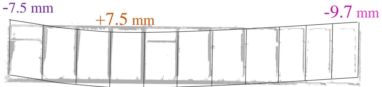
**Figure 38: Deviation pattern in the form of bowing along the lengths of the roof frame (not to scale)**
