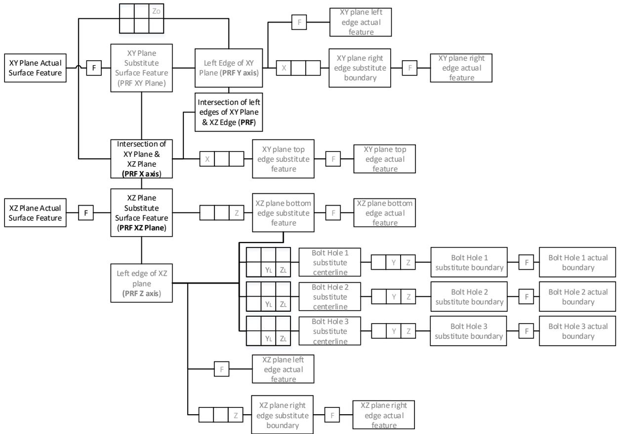
**Figure D30: Part Diagram for Tie-in Plates**
