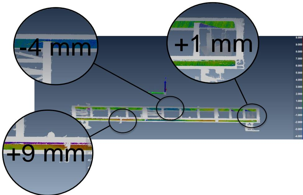
Figure 34: Plane analysis output using PolyWorks® for both lengths of the floor frame of interest
