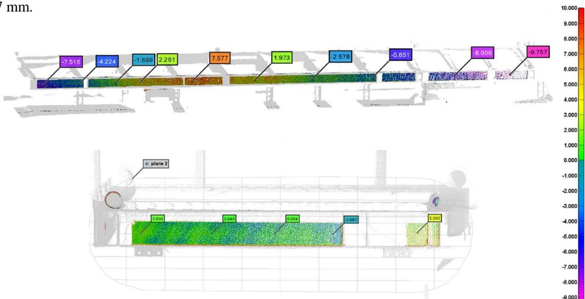
Figure 37: Plane analyses outputs using PolyWorks® for length and width of roof frame (deviations in mm)
