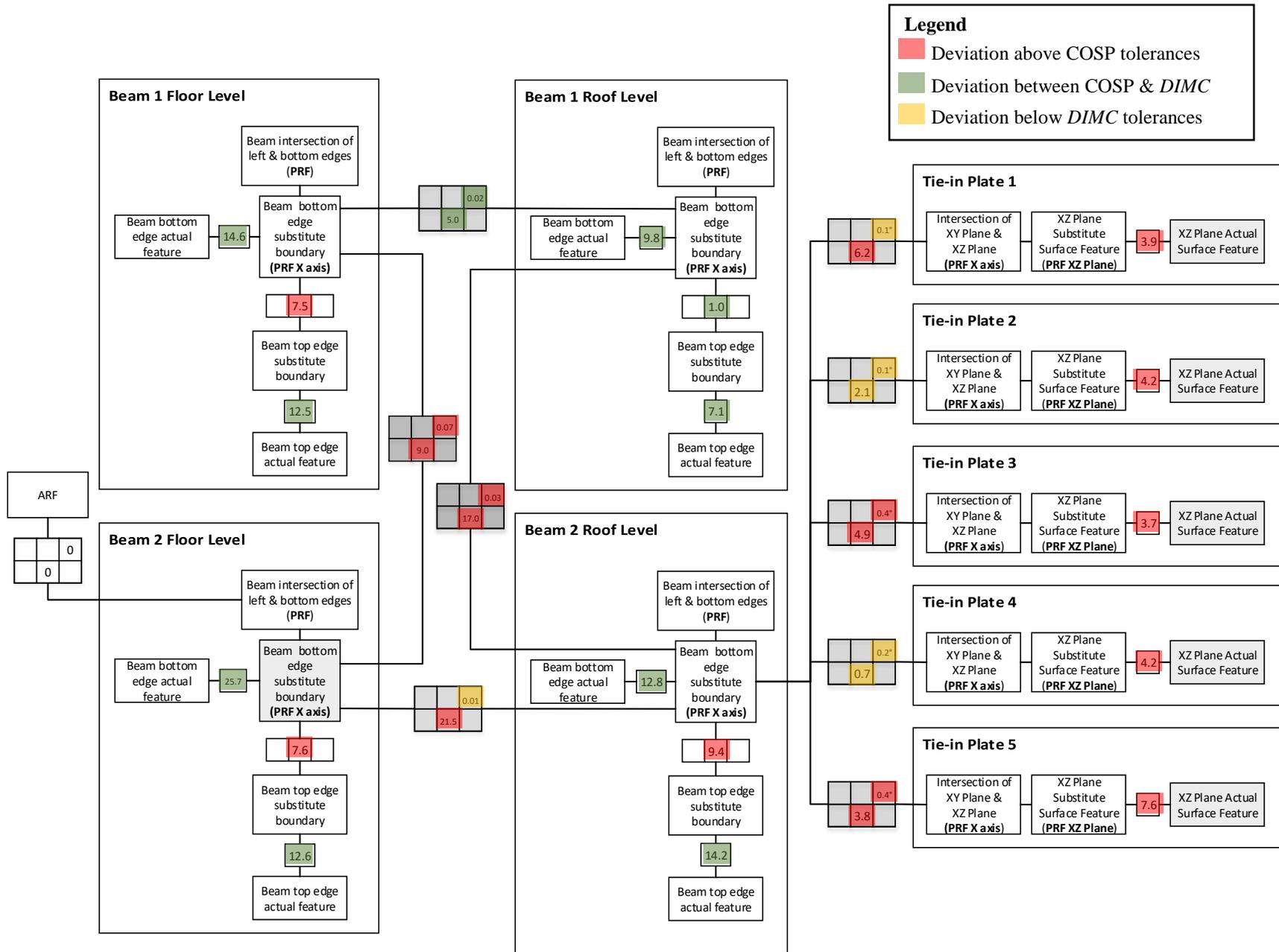
Figure 61: Comparison of deviations with respect to both tolerance maps employed in the second case study for assessing process capabilities
