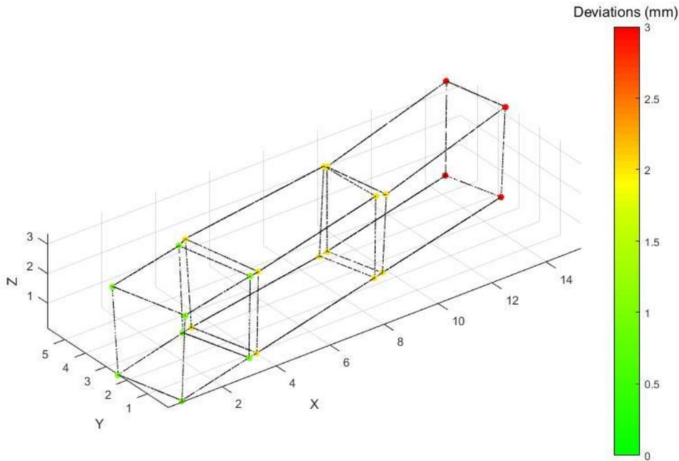
**Figure 54: Deviation analysis using MATLAB® code and surveying of 24 key locations on the module in order to quantify dimensional variability associated with transportation loading.**
