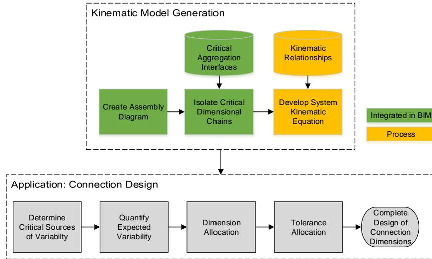
**Figure 62: Overview of the proposed method for kinematics chain-based dimensional variation analysis.**
