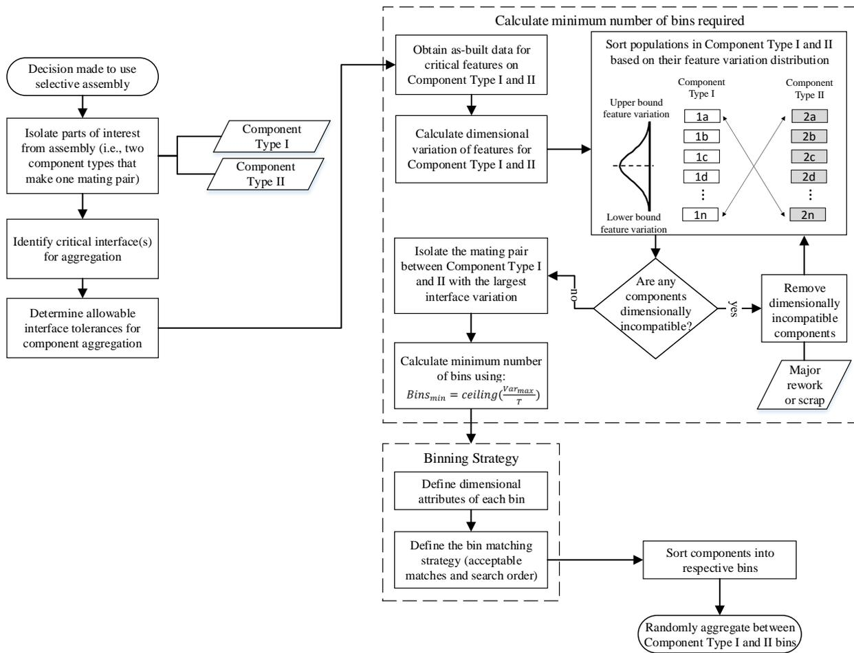
Figure 76: Framework of proposed use of selective assembly in modular construction
