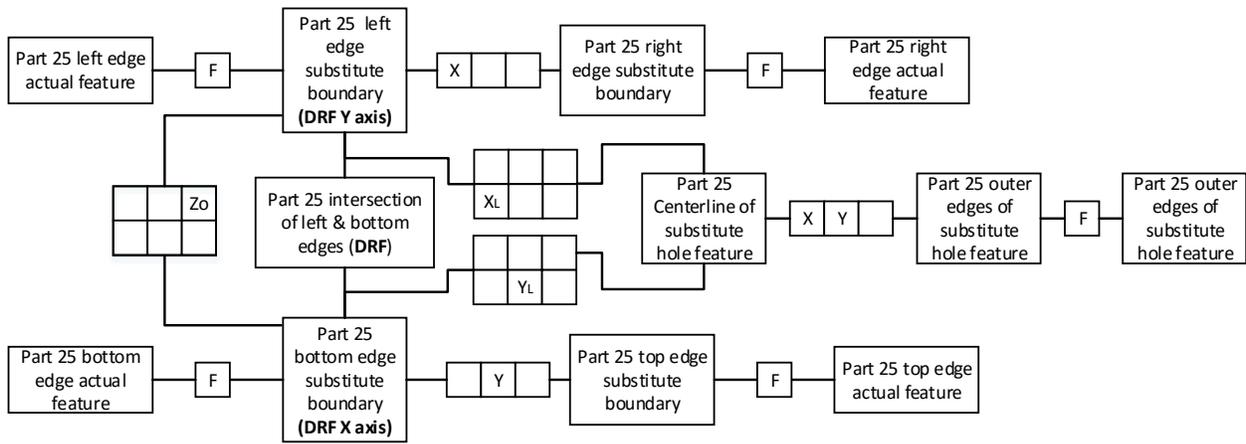
**Figure D6: Part Diagram for Part 25**
