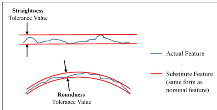
**Figure A3: Depiction of form tolerances of a line (straightness and roundness)**
