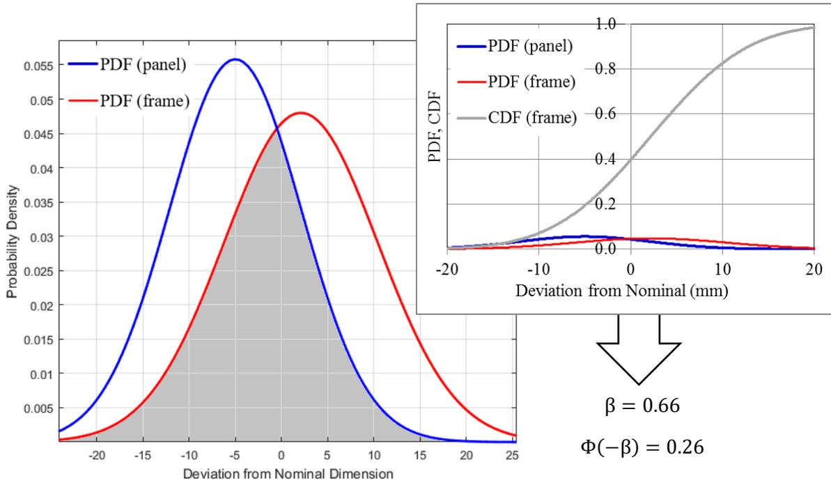
**Figure 41: Comparison of probability distributions for panel and frame dimensions. Probability of non-compliance equal to 26% based on reliability index calculation. Dimensions in mm.**
