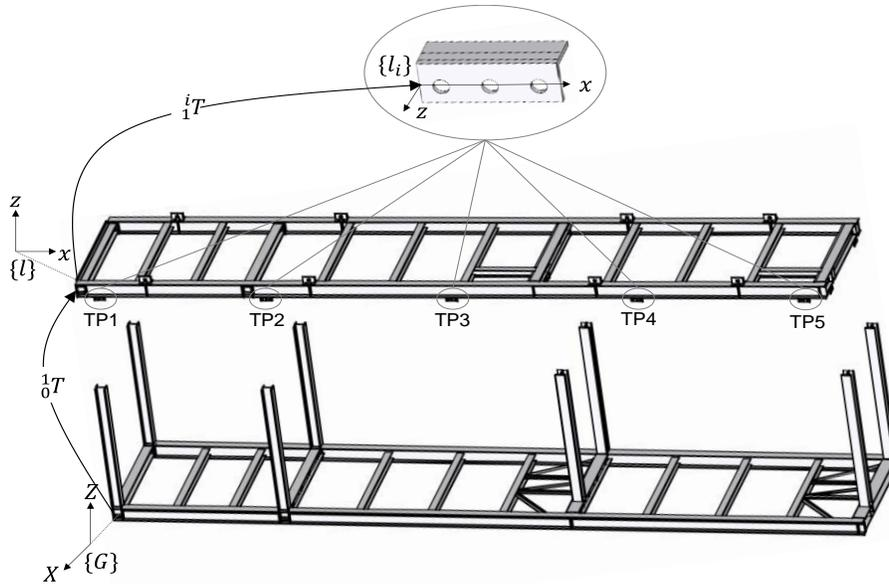
**Figure 68: Kinematics chain and transformations for representing critical features in the local  $\{L_i\}$  and global  $\{G\}$  coordinate systems.**
