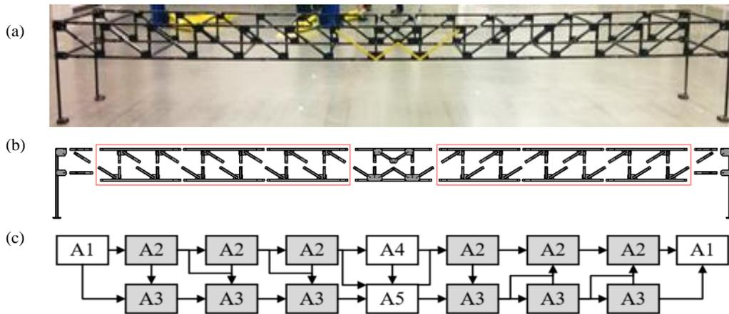
Figure 77: (a) Fully assembled steel bridge, (b) deconstructed single truss, (c) assembly diagram of single truss showing the five main assembly types.
