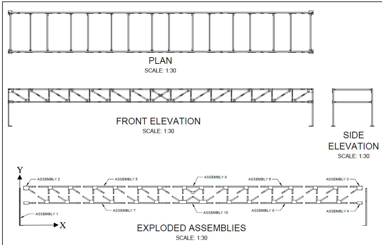
**Figure D1: Scale Drawing of Bridge Truss**
