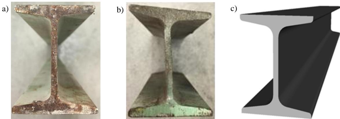
**Figure 17: Two S75x8 beams compared with a BIM model in order to assess mill tolerance compliance and to quantify geometric distortion during fabrication. Beam 1 (a) and beam 2 (b) are compared with (c) BIM element.**
