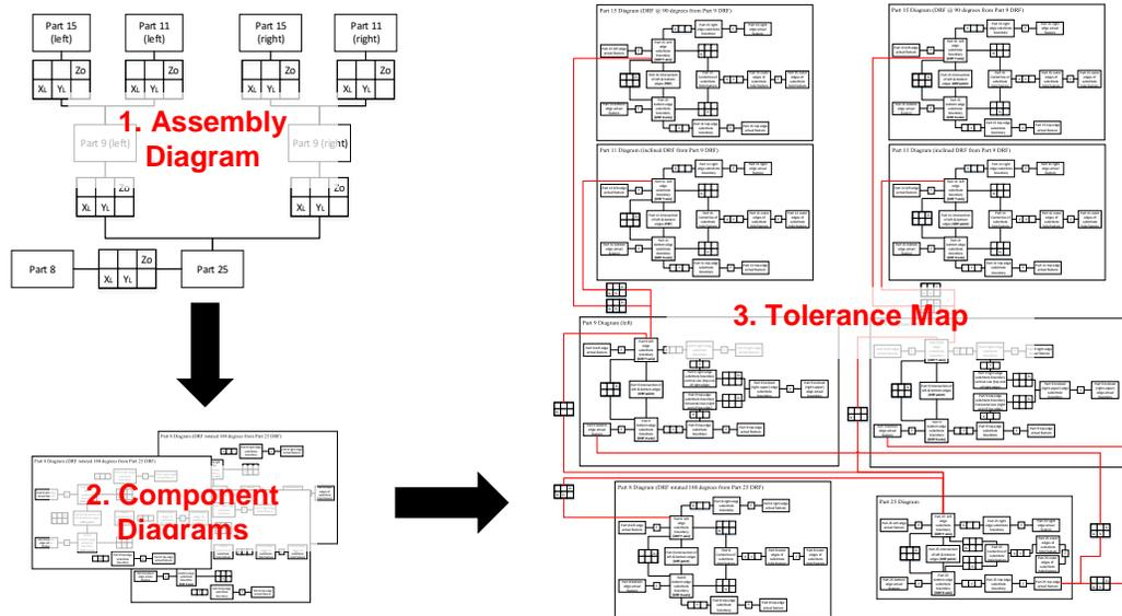
**Figure 59: Example of steps involved for creating a tolerance map: (1) create the assembly diagram, (2) create diagrams for each component and (3) amalgamate all component diagrams into the assembly diagram to obtain the overall tolerance map**
