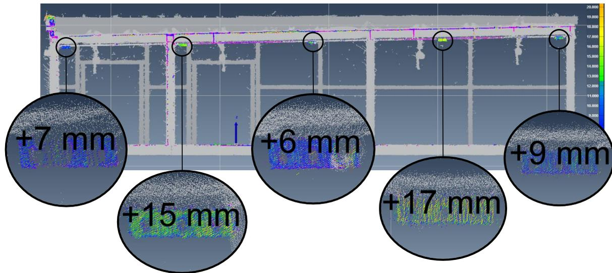
**Figure 44: Plane deviation analysis using PolyWorks® to quantify dimensional variability associated with tie-in plates with respect to the overall module datum (specified on the floor frame)**
