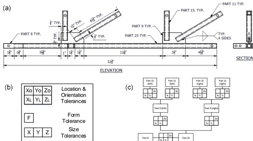
**Figure 58: Example of steps involved with creating an assembly diagram for a single structural assembly. (a) A dimensioned drawing for an assembly is broken down into its sub-components using (b) Geometric Dimensioning and Tolerancing notation to create (c) an assembly diagram.**
