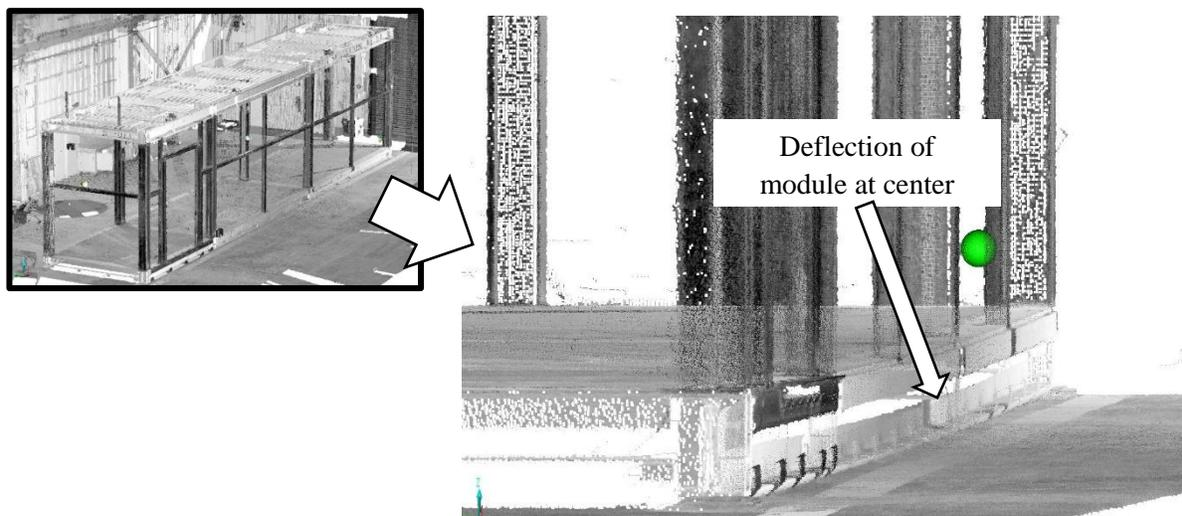
**Figure 50: Demonstration of the module elastic deflection while sitting on only four cribbing supports at the corners.**
