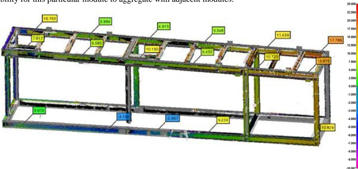
Figure 42: Deviation analysis output using PolyWorks® for the overall module assembly (note: concrete panels are not shown or assessed in this analysis, all deviations in mm)
