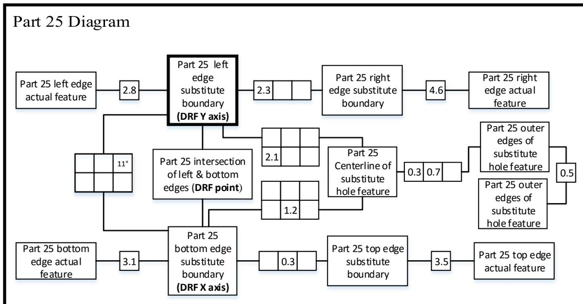
**Figure D16: Tolerance Map (above) and Deviation Map (below) for Part 25**
