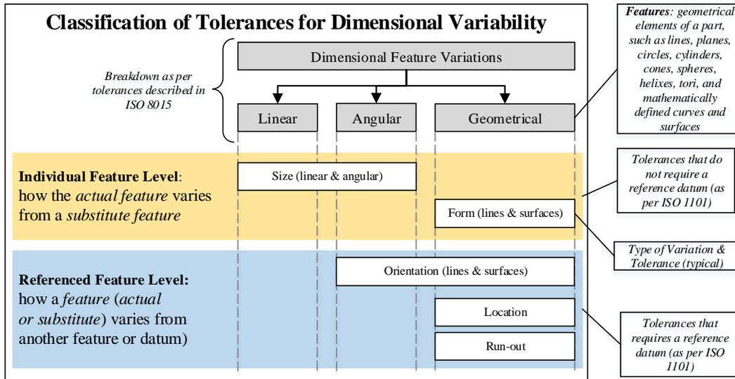
**Figure 8: Classification of dimensional variability and corresponding tolerances in manufacturing**
