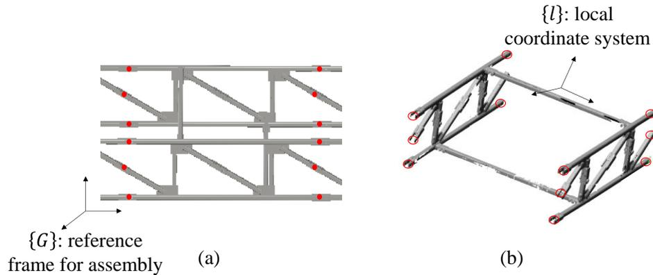
**Figure 89: Critical points extraction for the 3D model (a), and laser scanned point cloud representing the as-built status (b).**
