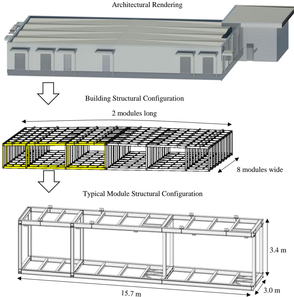
**Figure 22: Case study to demonstrate how dimensional variability accumulates throughout an offsite construction assembly during the life cycle.**
