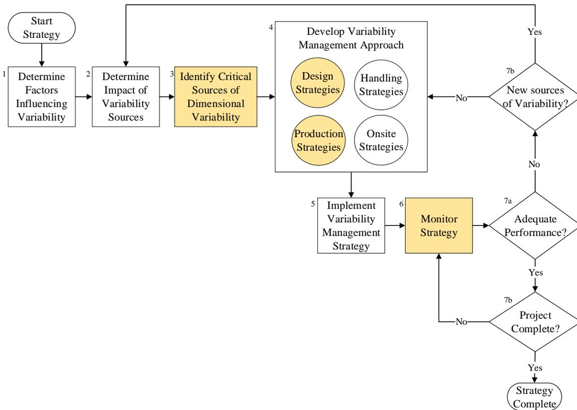
**Figure 9: Proposed framework for managing dimensional variability throughout the construction lifecycle (manufacture, fabrication, aggregation, transportation, handling and erection) of a modular construction project. New developments made in this thesis are highlighted in yellow.**
