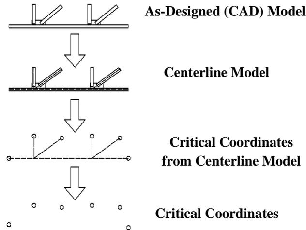
**Figure 79: Process of extracting critical coordinates from original as-designed model**
