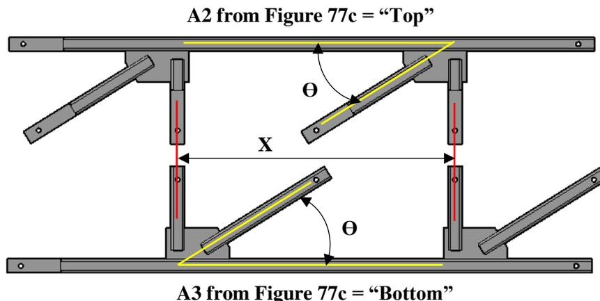
Figure 78: Repetitive assembly pair in case study, with critical interface dimensions as  $\Theta$  (yellow) and  $X$  (red)
