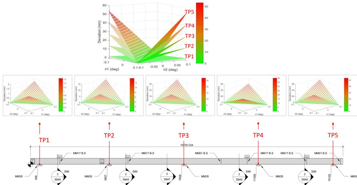
**Figure 71: Propagation of dimensional variation along the roof frame for different tie-in plates. As seen, tie-in plates further from the datum have larger impacts. Using kinematics chains, thorough analyses are possible using mathematical relationships between different components.**
