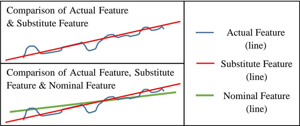
**Figure A2: Comparison of actual feature, substitute feature and nominal feature**
