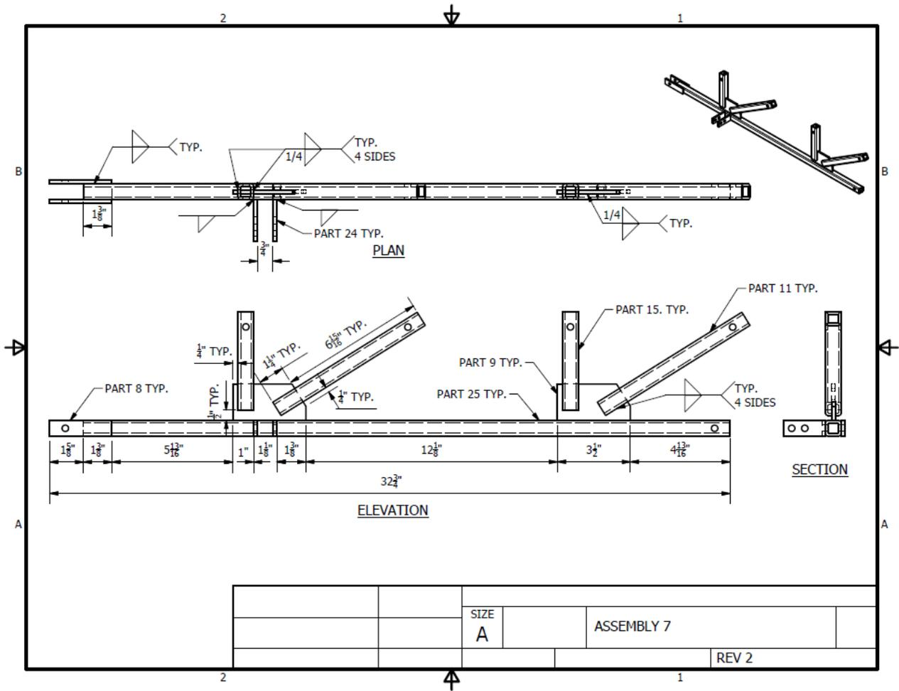
Figure D3: Shop Drawing of Assembly 7
