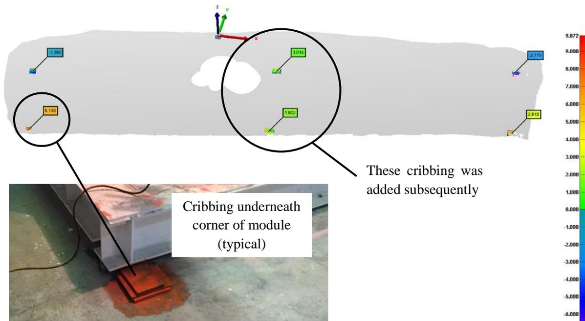
**Figure 49: Shop floor cribbing conditions: first condition comprised only the outer four supports, however during the project two additional cribbing supports were added in the center. This figure also shows the output of a plane deviation analysis using PolyWorks® of the dimensional variability associated with the vertical elevation of the cribbing (deviations are in mm).**
