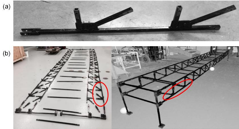
**Figure 57: Structural component used to demonstrate creation of a tolerance map. (a) Structural assembly of component. (b) Location of component in overall modular bridge.**
