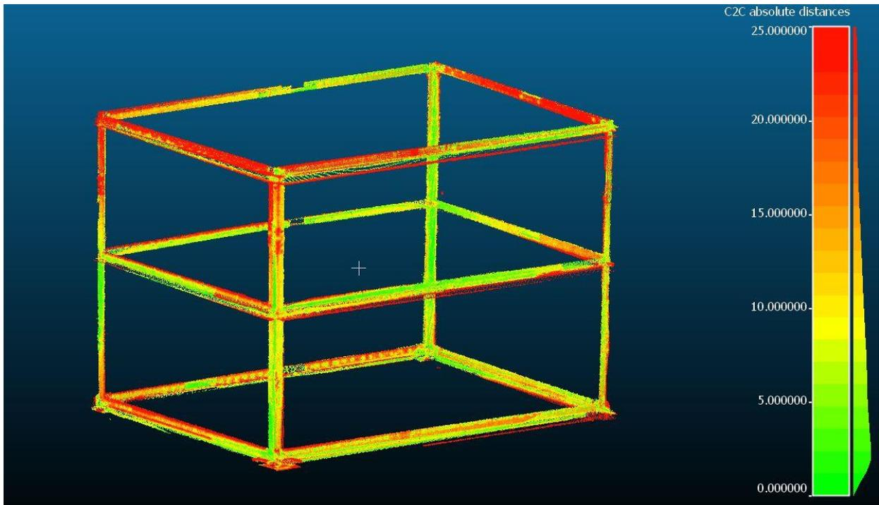
**Figure B4: Deviation analysis output for Trimble® GX 3D Laser Scanner**
