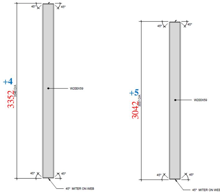
**Figure 43: Comparison of nominal dimensions for length of columns to extracted as-built dimensions from the point cloud (note: as-built dimensions are in red, and deviations with respect to the nominal dimensions are displayed in blue with a plus/minus value). Dimensions in mm.**
