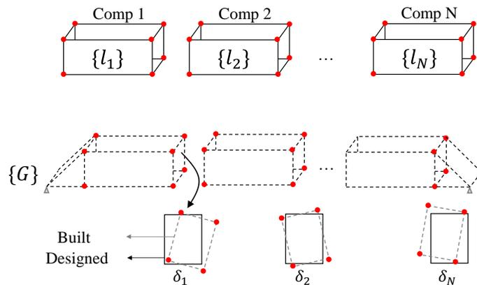
**Figure 86: Hypothetical example for optimizing the assembly plan using approach II (rework avoidance). For each segment, the component which is closest to the as-designed status is picked from the remaining components until the assembly plan is complete ( $\delta_i$  is the minimum deviation for the remaining components).  $\{l\}$  and  $\{G\}$  are local and global coordinate systems respectively.**
