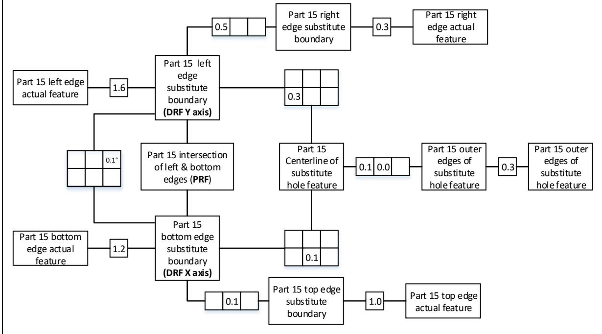
Figure D20: Tolerance Map (above) and Deviation Map (below) for Part 15 (left)
