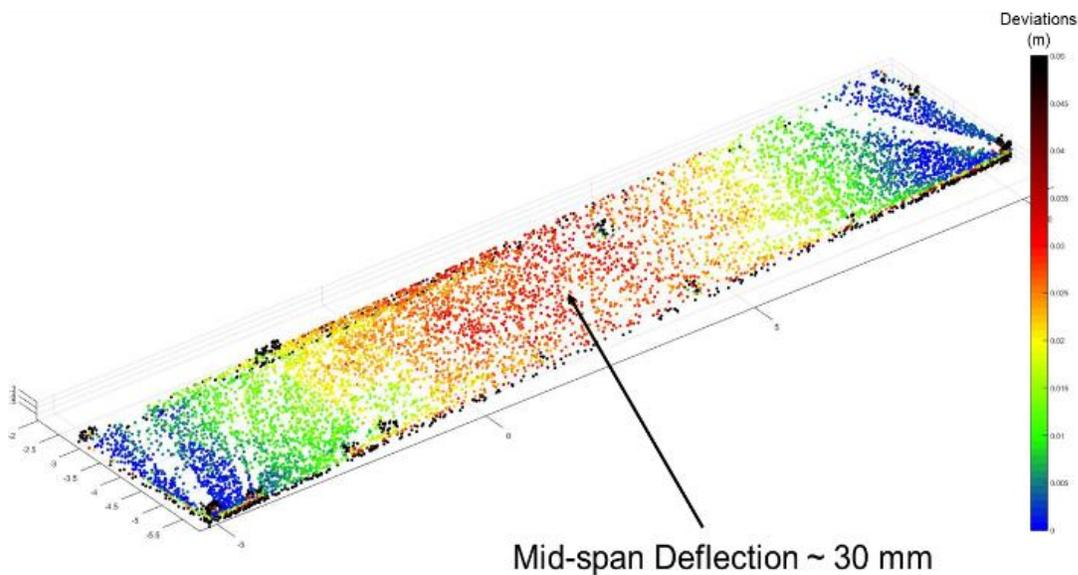
**Figure 51: Scan-to-scan analysis of the module sitting on the BLUCO framing table and on 4 shop floor cribbing supports.**
