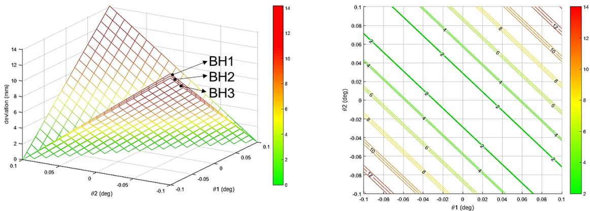
**Figure 72: Results for laser-based DVA of the case study. Deviation surfaces and contour lines for the bolt holes (BH) are illustrated. The results are shown for the tie-in plate 2 (TP2) illustrated in Figure 68.**
