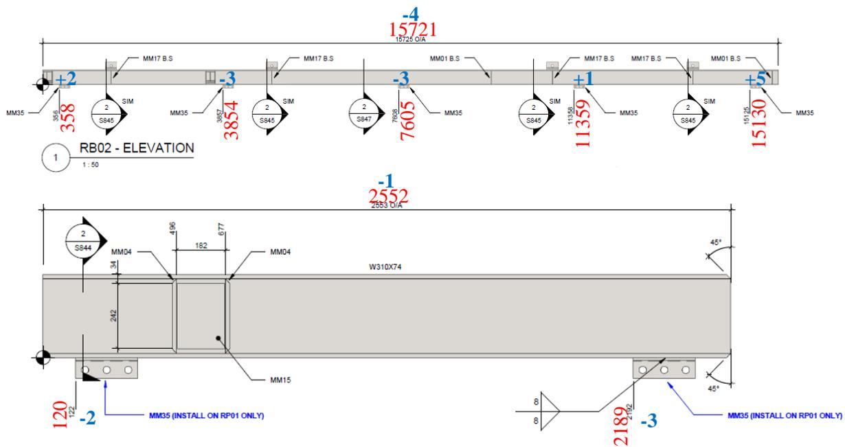
**Figure 39: Comparison of nominal dimensions for overall length, width and location of tie-in plates to extracted as-built dimensions from the point cloud for the roof frame (note: as-built dimensions are in red, and deviations with respect to the nominal dimensions are displayed in blue with a plus/minus value, all dimensions in mm).**
