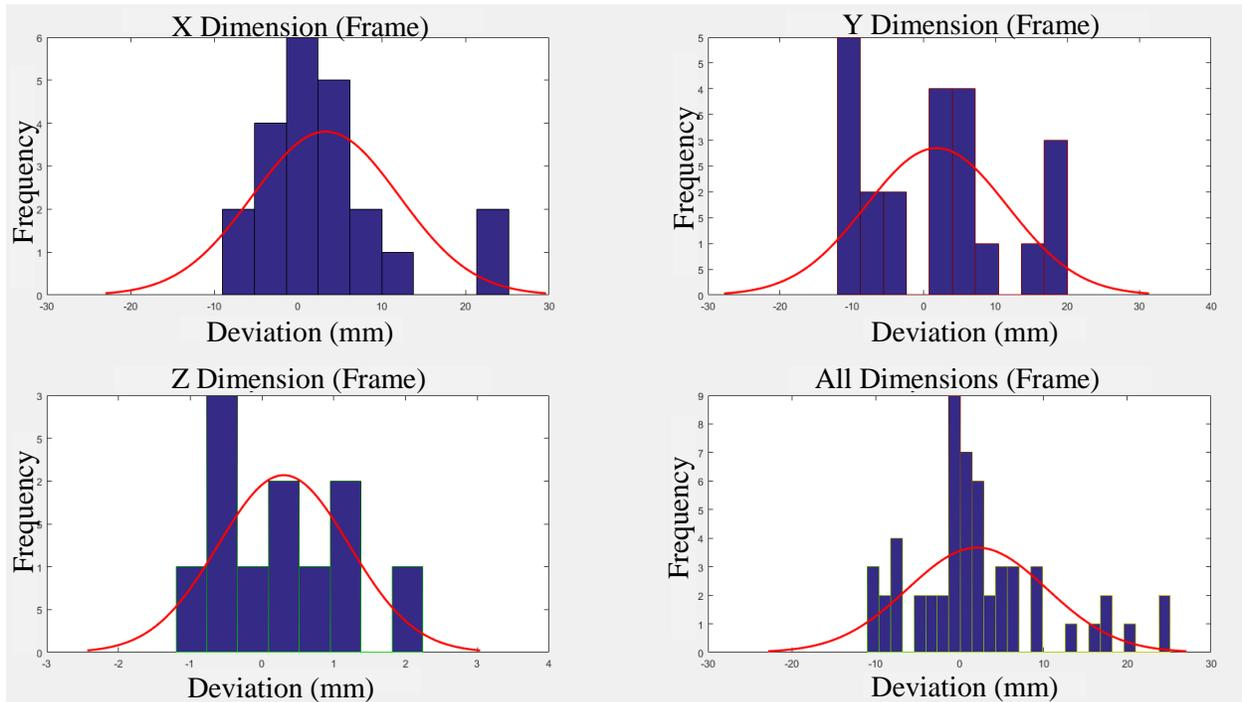
**Figure 32: Histogram plots for the dimensional variability of frame as-built dimensions.**
