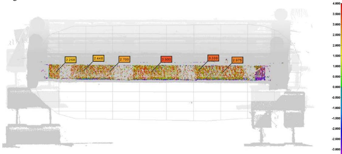
Figure 33: Plane analysis output using PolyWorks® on sample width of floor frame (deviations in mm)
