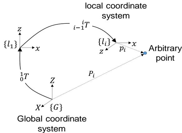
**Figure 69: Relationship between positions in the local ( $p_i$ ) and global ( $P_i$ ) coordinate systems. Coordinate systems are defined based on D-H convention.**
