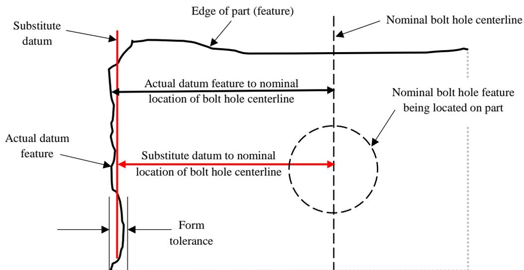
**Figure A8: Depiction of form tolerance for substitute datum features**
