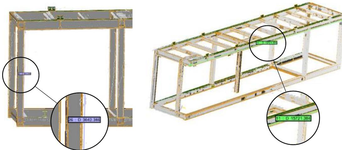
**Figure 74: Sample extracted dimensions (in mm) from 3D point cloud model using PolyWorks®**
