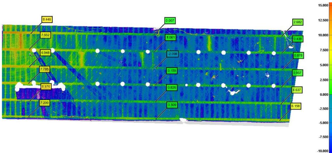
**Figure 47: Plane analysis output using PolyWorks® for dimensional variability of BLUCO framing system (deviations are in mm)**
