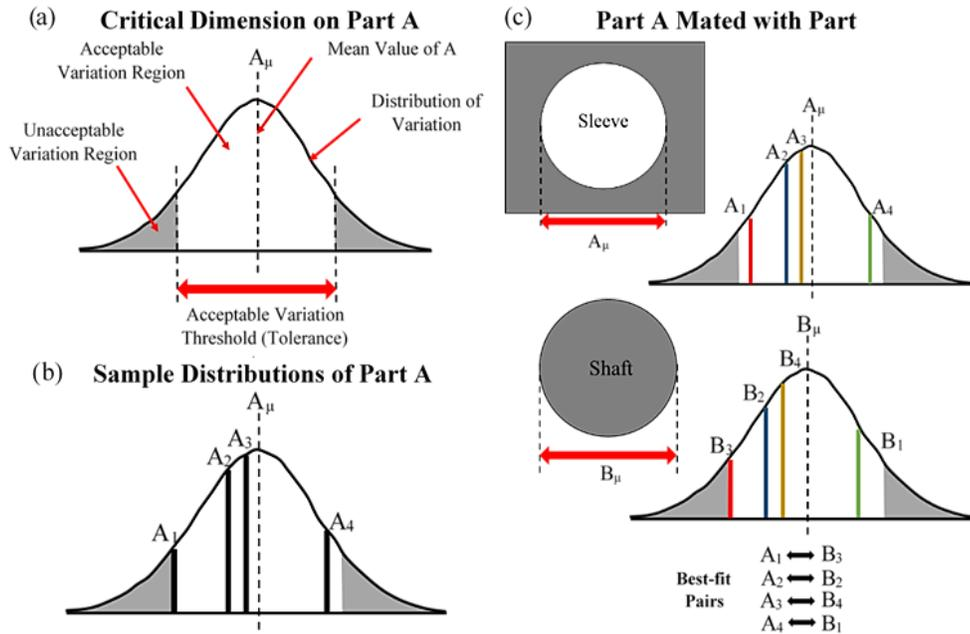
**Figure 75: Demonstrating the concept of selective assembly: (a) dimensional distribution of critical feature for aggregation, (b) sample distributions of feature and (c) optimal matching of sleeve and shaft parts based on the distribution of critical aggregation features.**
