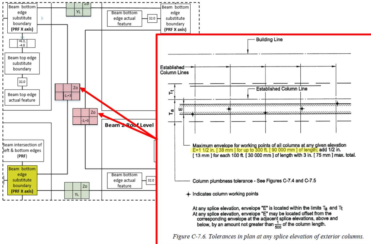
**Figure D32: Derivation of Orientation Tolerances in Z direction between Beams in Case Study 2**
