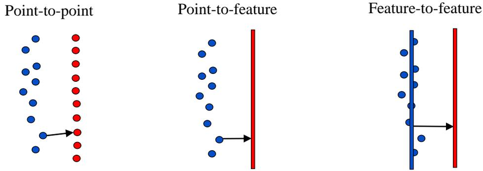
**Figure 15: Comparison types between two data sets in proposed deviation analysis method (e.g., blue data set represents as-built state, and red data represents as-designed state)**
