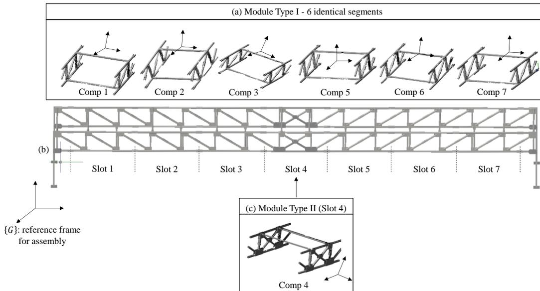
**Figure 88: Assembly planning for Case I. (a) 6 interchangeable modules of type I are scanned and critical points are extracted (see Figure 89). (b) Critical points in the 3D models are extracted at each slot. (c) Module type II is installed in the Slot 4, which makes a constraint in the assembly planning and the optimization problem involved.**
