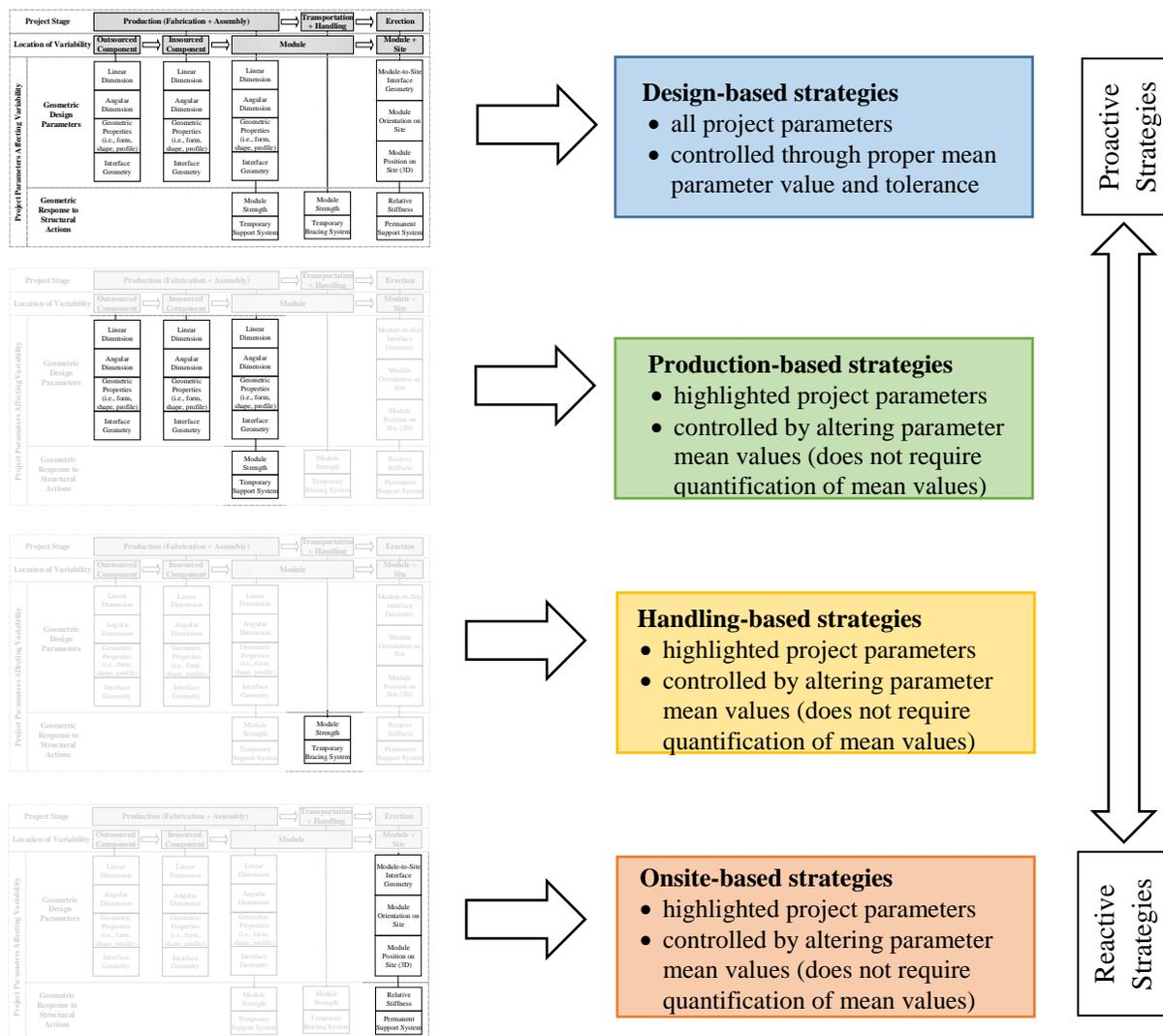
**Figure 11: Scope of project parameters which relate to design-based, production-based, handling-based or onsite-based dimensional variability management strategies**
