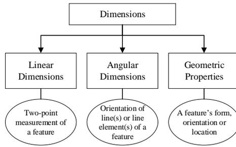
**Figure 12: Breakdown of dimensional tolerances as presented in (ISO 1985)**
