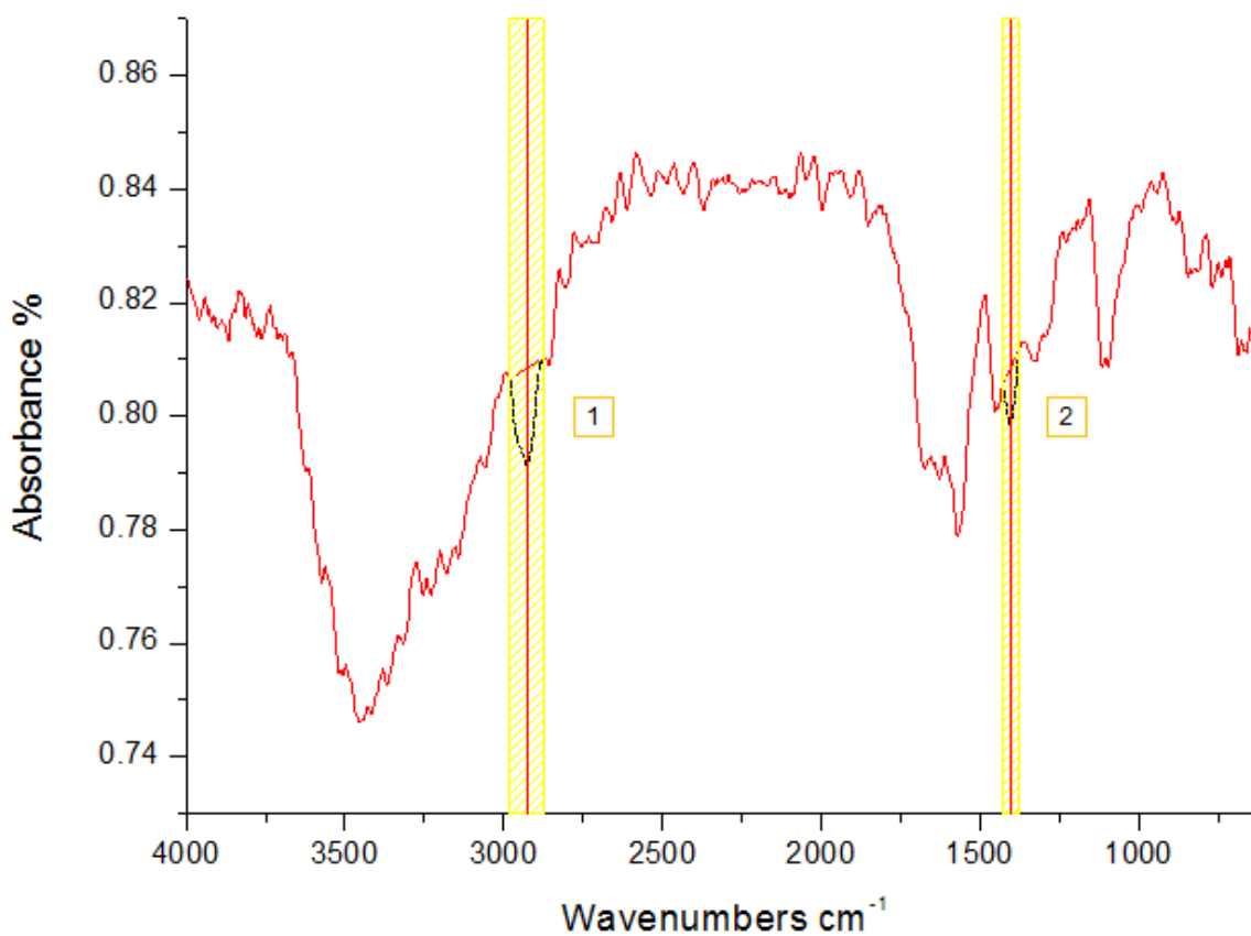
Figure 5- 4 Chosen band and method of calculation of relative peak area. The spectrum is 55% NaA monomer concentration.
