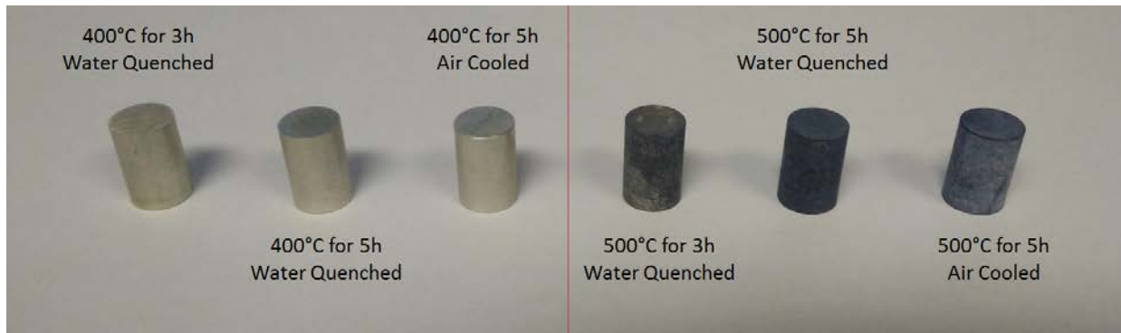
Figure 4-25: Compression samples homogenized under various conditions.
