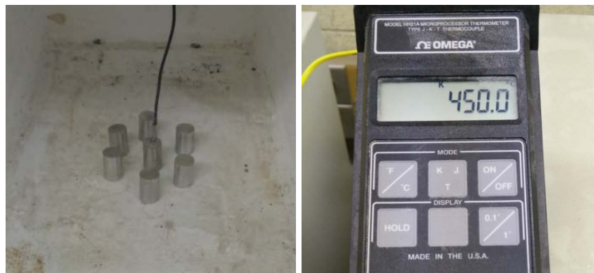
Figure 3-11: Temperature calibration for homogenization procedure.
