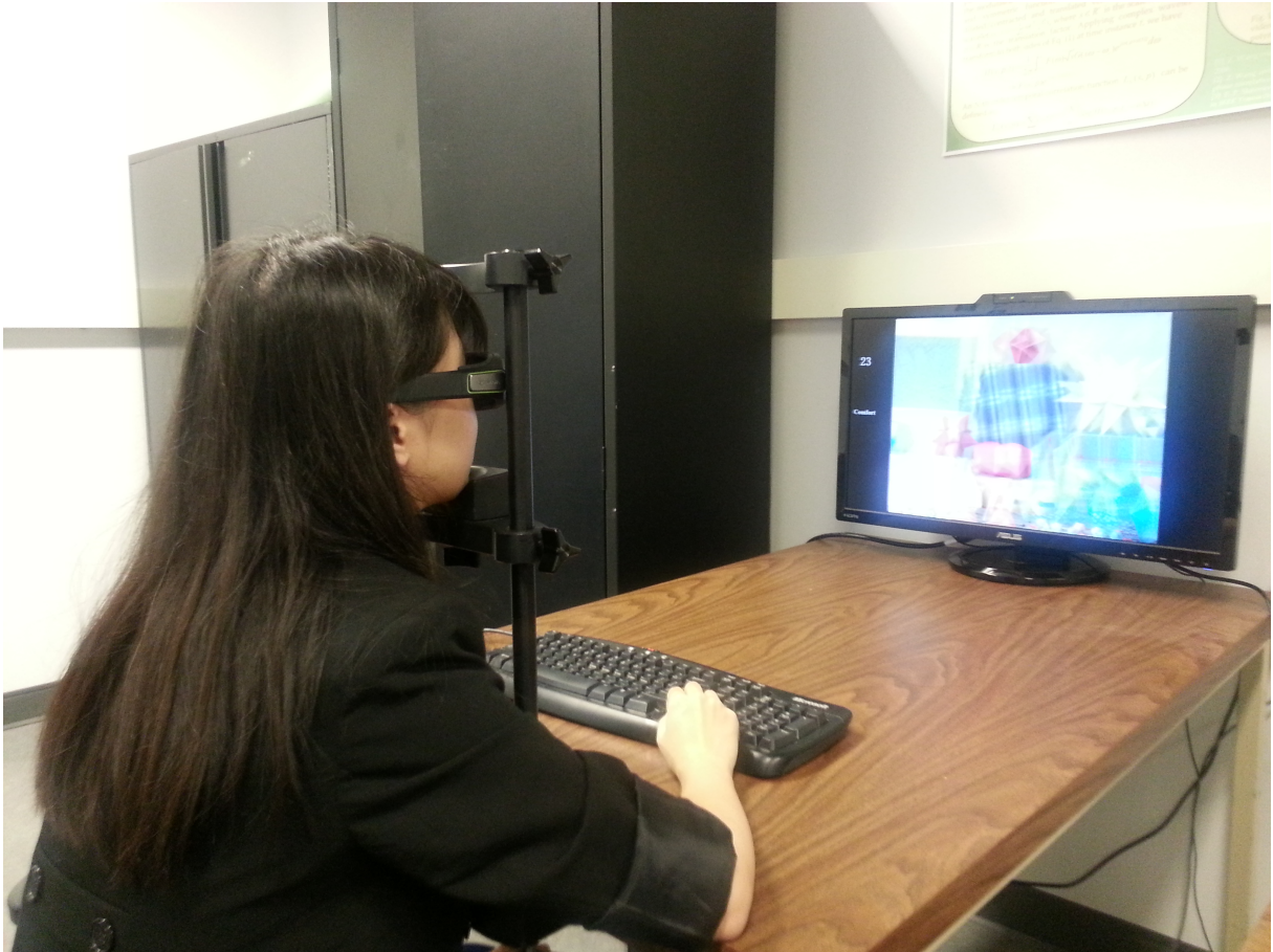
Figure 3.4: Experimental setup: the subject is facing the 3D LED monitor with active shutter glasses using a holder to control the viewing distance.
