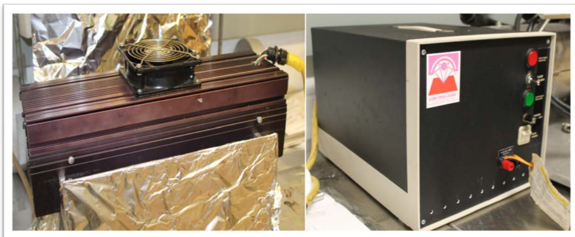
Figure 3.4 – UV Lamp and its Controller with Intensity Set Points
