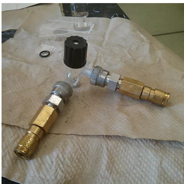
Figure 6-1 - Reaction vessel for the acid treatment of electrodes. The two quick connects serve as the gas flow inlet and outlet. The top is fitted with an air-tight septum to allow for injection of the acid with minimal air exposure.
