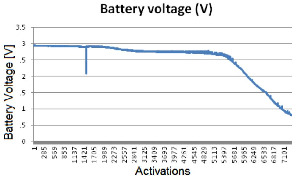
FIGURE 4-6: BATTERY VOLTAGE DROP FOR AN A/I RATIO OF 1.0
