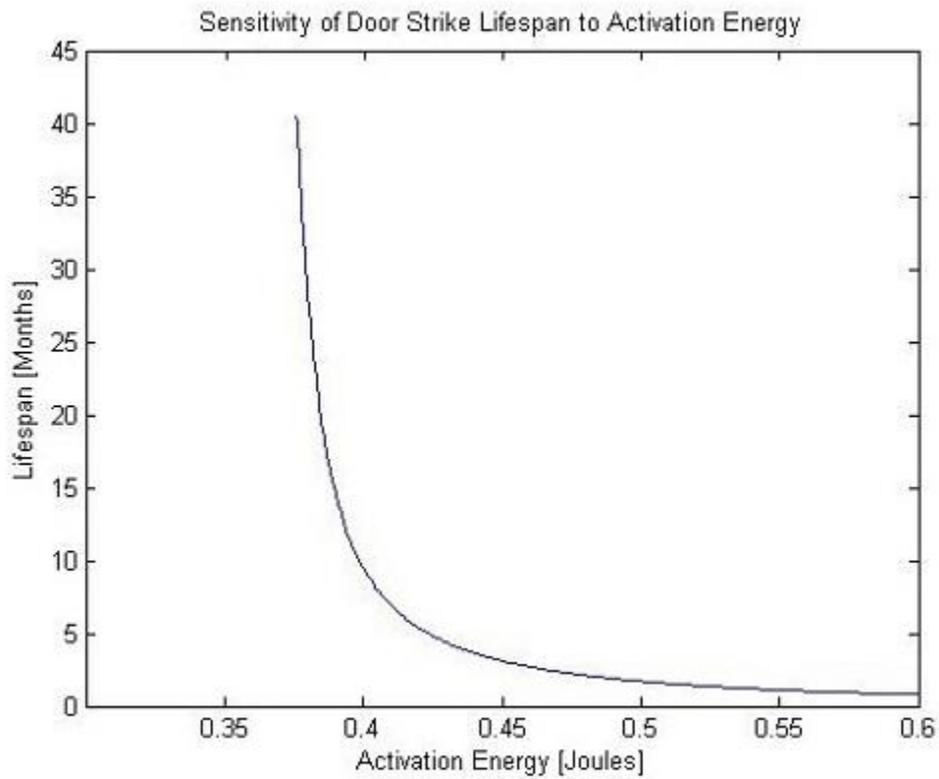
FIGURE 3-6: SENSITIVITY OF DOOR STRIKE LIFESPAN TO ACTIVATION ENERGY
