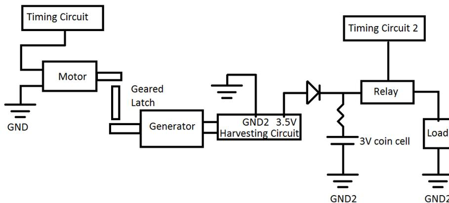
FIGURE 4-3: HYBRID DOOR STRIKE EXPERIMENTAL DIAGRAM
