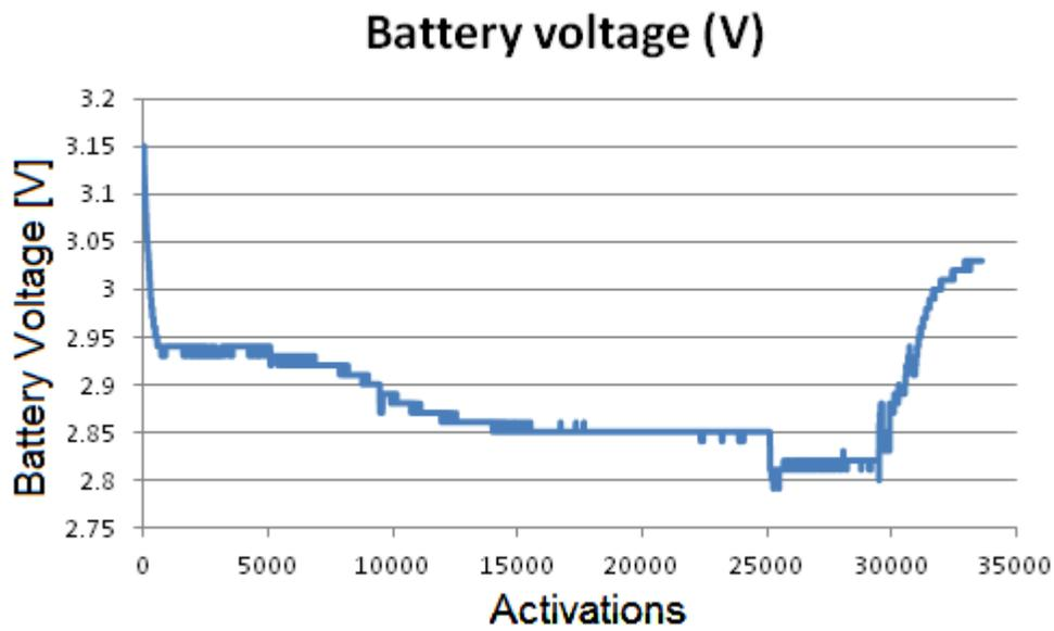
FIGURE 4-8: BATTERY VOLTAGE DROP FOR AN A/I RATIO OF 0.1
