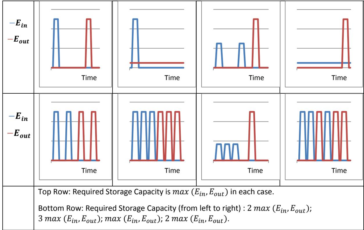
FIGURE 3-1: POSSIBLE ENERGY FLOW CASES IN A SYSTEM WITH EITHER CONSTANT OR IMPULSIVE INPUT AND OUTPUT
