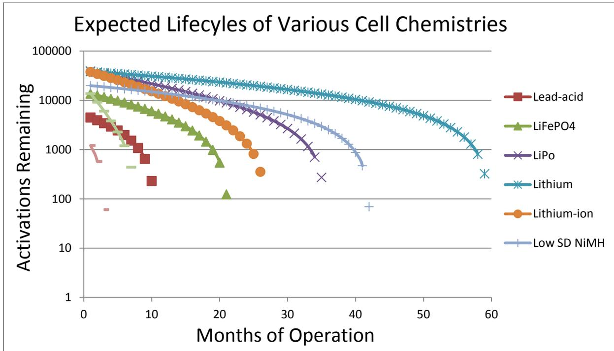
FIGURE 3-2: EXPECTED LIFECYCLES OF VARIOUS CELL CHEMISTRIES. 150 ACTIVATIONS PER MONTH, 40% HARVESTING EFFICIENCY.
