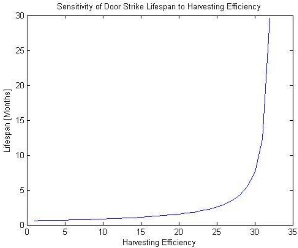
FIGURE 3-3: SENSITIVITY OF DOOR STRIKE LIFESPAN TO HARVESTING EFFICIENCY
