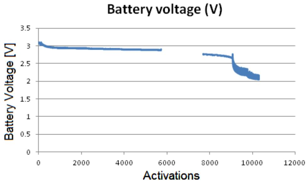
Figure 4-7: Battery Voltage Drop for an A/I Ratio of 0.5
