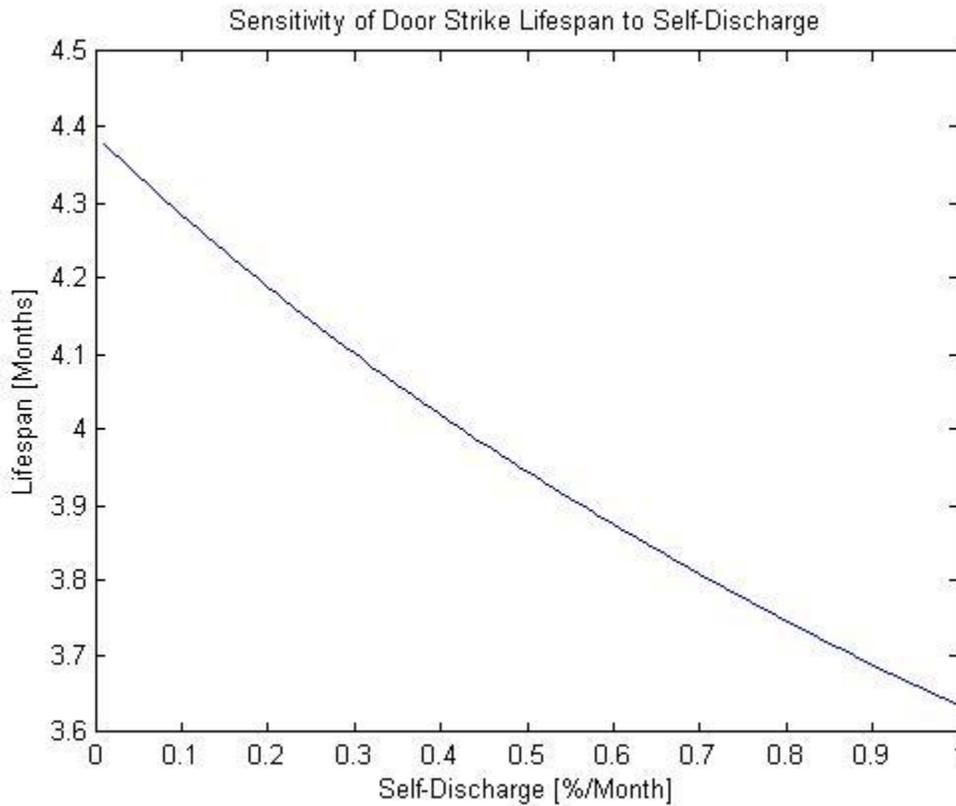
FIGURE 3-9: SENSITIVITY OF DOOR STRIKE LIFESPAN TO PASSIVE BATTERY LEAKAGE
