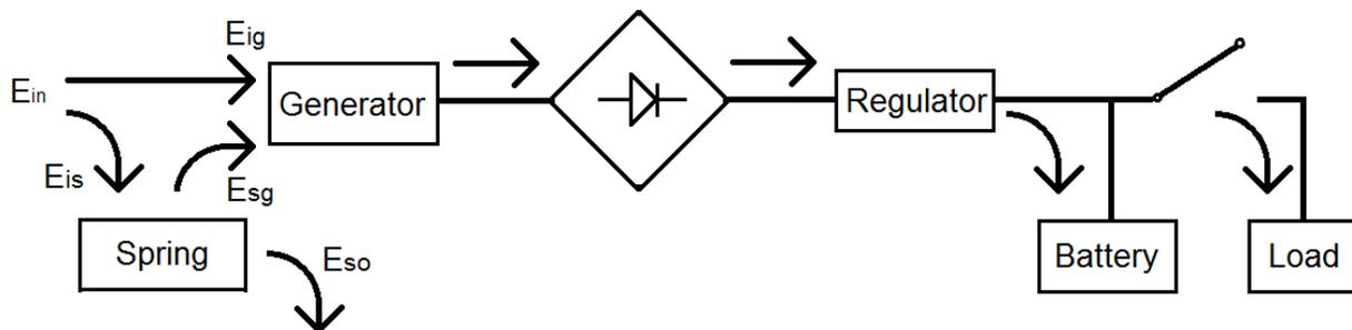
FIGURE 4-1: ENERGY FLOW DIAGRAM OF HYBRID E-STRIKE
