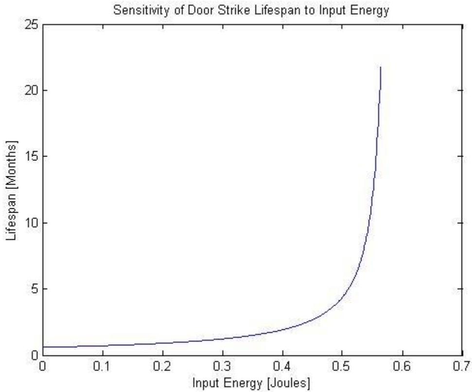
FIGURE 3-5: SENSITIVITY OF DOOR STRIKE LIFESPAN TO INPUT ENERGY
