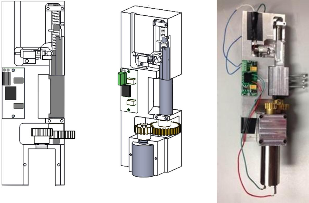
**FIGURE 4-4: E-STRIKE TESTING APPARATUS**
