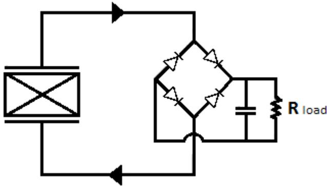
FIGURE 1-2: STANDARD MODEL OF VIBRATION ENERGY HARVESTING
