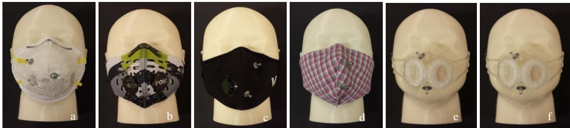
Figure F-1. Respiratory dust masks used in this study from left to right: a , b , c , d , e , and f ) replacing the filter of the commercial respiratory mask e with the fabricated nanofibrous filters
