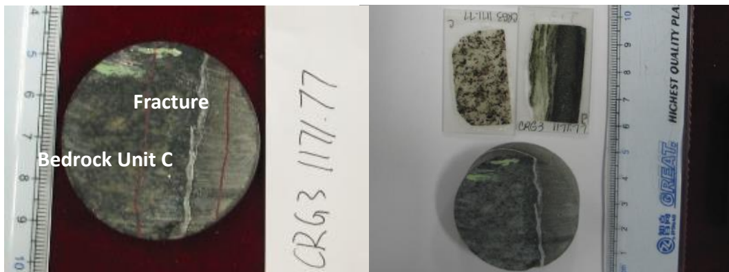
Figure 9f. Hand specimen showing different bedrock types separated by calcite filled fracture in a thin section from borehole CRG3 at 1171.77 m depth.
