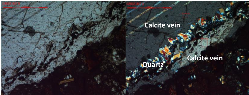
Figure 9d. Quartz vein enclosed by calcite veins in borehole CRG3 at 307.9 m, left photo is under plane light and right photo is under polarized light.
