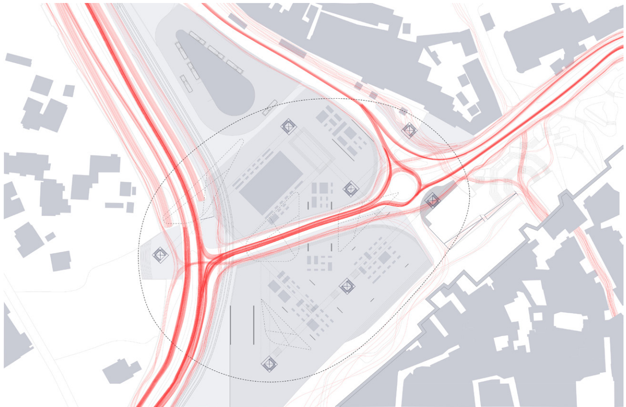
Fig. 3.52 Ground Conditions. Diagram 06 - Traffic / Site Circulation. Lines in darker red represent vehicular traffic and those in beige represent human circulation. The density, and composite thickness, of the lines correlates to the speed and consistency of movement along that given route. As the final layer of the composition the access cores, roof line and overhead conditions are overlayed on the ground condition.
