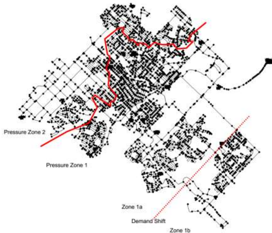
Figure 2.1: City X WDN model components; pressure zones and demand shift highlighted
