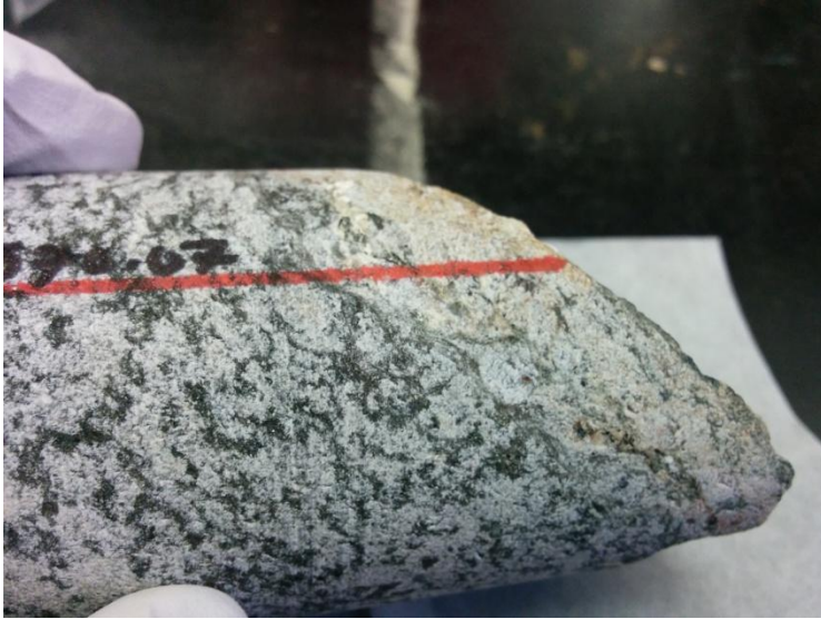
Figure D-6. DH-GAP04 570.07 m. Photo of alteration along fracture at 570.07m. Visually, chlorite was also present in sample.
