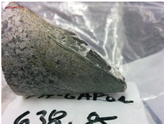
Figure D-9. DH-GAP04 638.85 m. Photo of alteration along fracture at 638.85 m.
