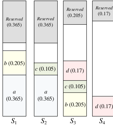
Figure A.1: Using RFI algorithm for placing a sequence of tenant replicas
