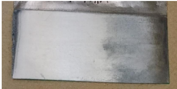
Figure 7 - Zinc deposited on a graphite foil via Hull cell experiment
