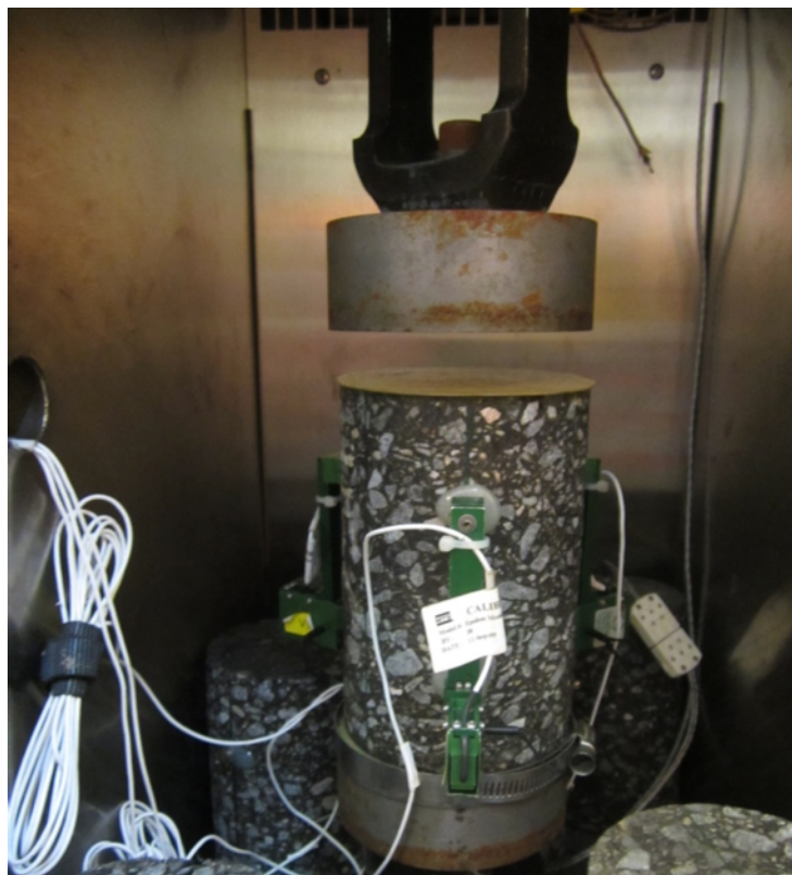
Figure 3-6 CPATT dynamic modulus test setup
