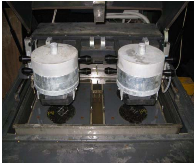
Figure 3-7 CPATT Hamburg wheel rut tester (HWRT)
