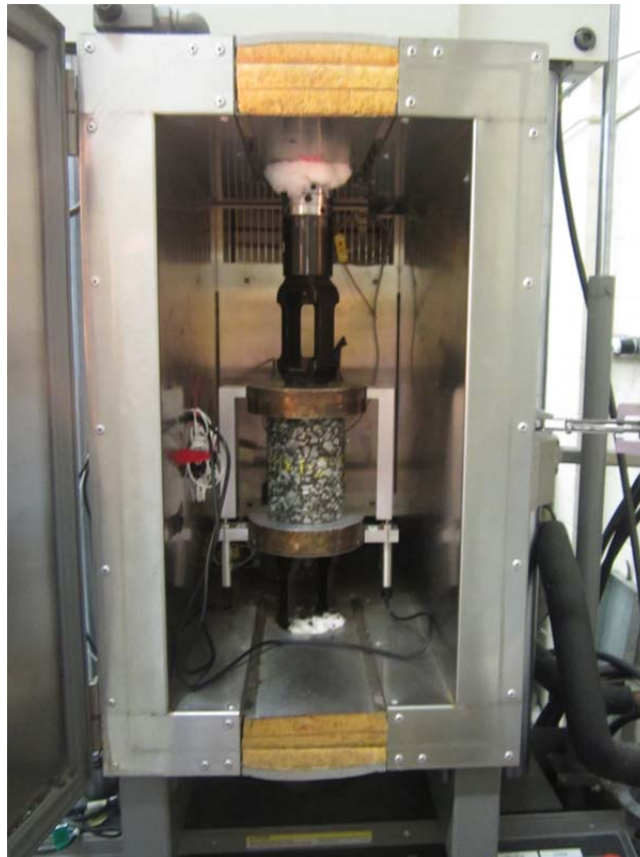
Figure 3-8 Flow number test setup
