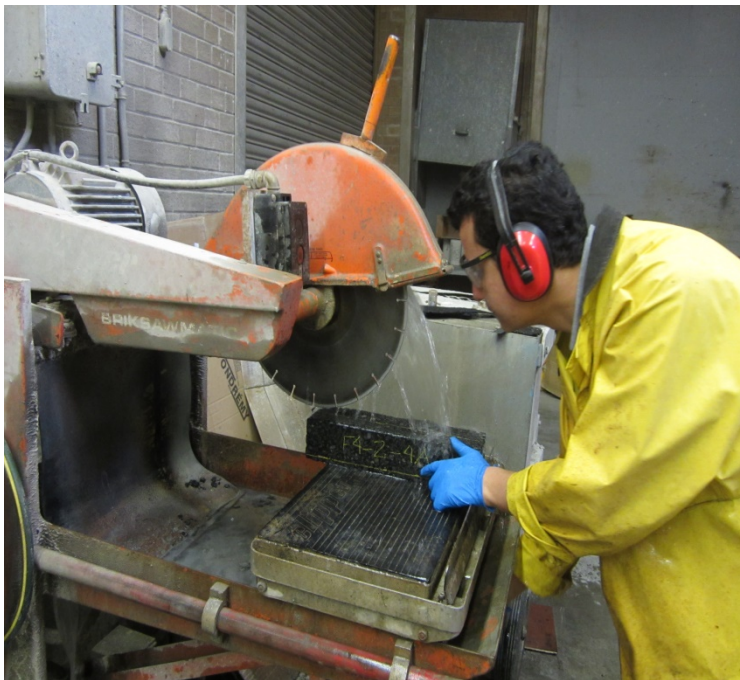
Figure 3-3 Saw cutting of fatigue asphalt beams
