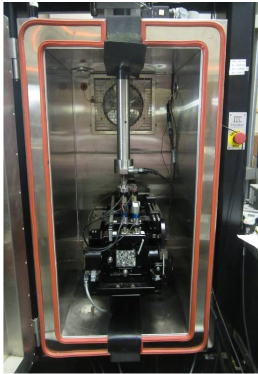
Figure 3-4 Temperature controlled CPATT flexural beam test setup
