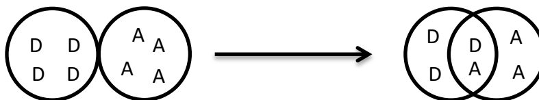
Figure 2: Illustration of the mixing between latex particles containing polymers labelled with a donor (D) and an acceptor (A) as the particles are annealed above the MFT.
