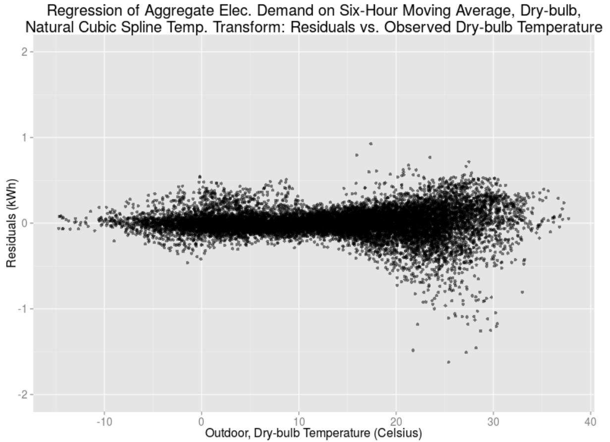
Figure 3.19: Residuals as a function of dry-bulb temperature observations, resulting from a comparison model using dry-bulb, six-hour moving average, and natural cubic splines to generate the temperature transformation matrix \mathbf{T} .
