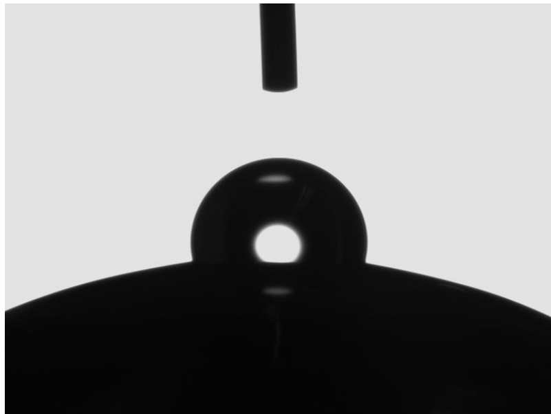
Figure 3-2. Image recorded by the Optical Contact Angle analyzer camera of the water droplet interacting with the lens surface.
