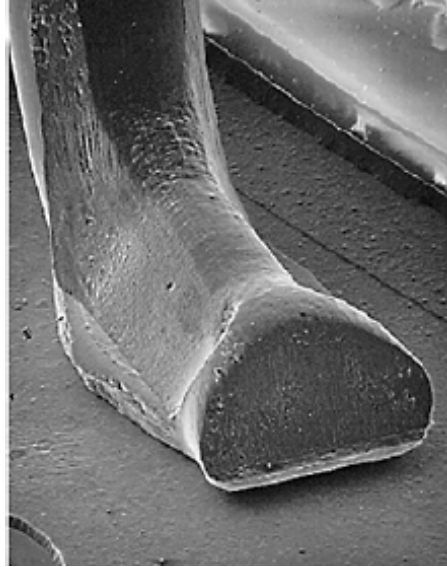
Figure 1.2: Close view of wedge bonding [5]
