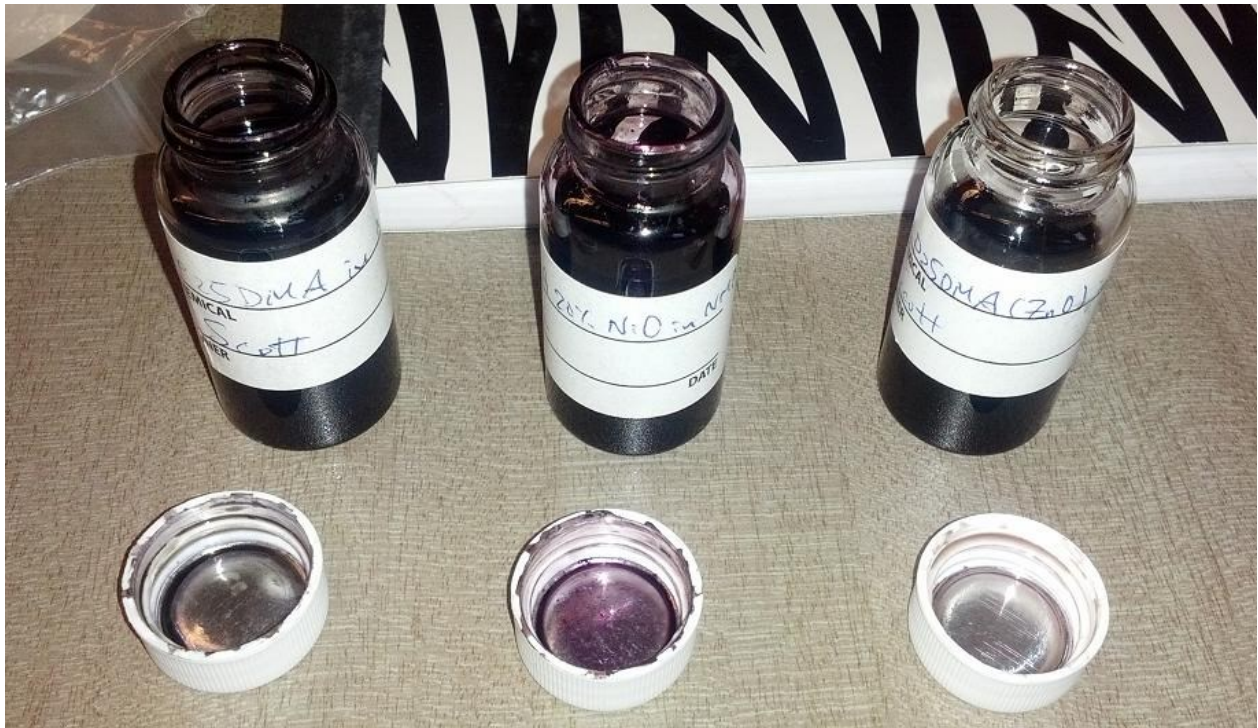
Fig. 3.4.5: Colour difference of the P25DMA family solutions (left - P25DMA, centre - P25DMA 20% NiO, right - P25DMA 20% ZnO).
