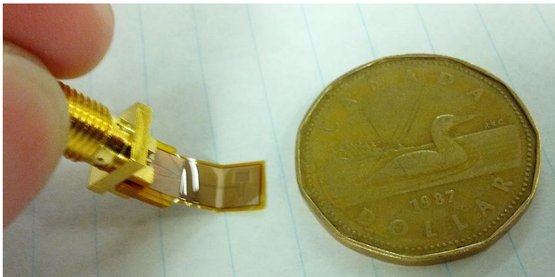
Fig. 5.4.3: Single RF resonant sensor on Kapton/SU-8 frame-flex substrate.
