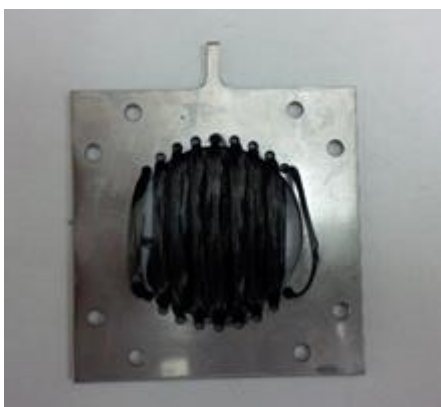
Figure 3.2: An anode module incorporated into the lab-scale MEC
