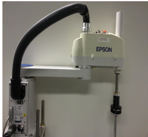
Figure 3.3: Force sensor mounted on the manipulator wrist.
