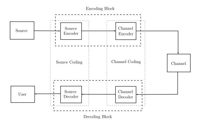
Figure 2.1: Point-to-point communication system model.
