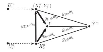
Figure 3.1: Correlated sources and phase incoherent causal cognitive multiple access relay channel (PI-CC-MARC).
