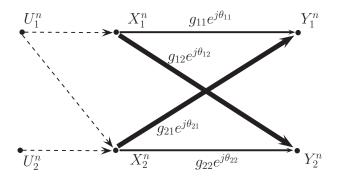
Figure 3.4: Correlated sources and phase incoherent noncausal cognitive interference channel
