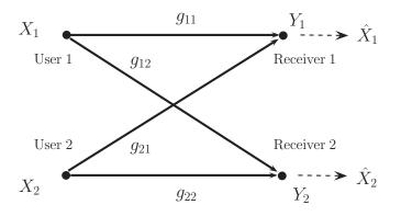
Figure 2.5: A 2-user Gaussian interference channel
