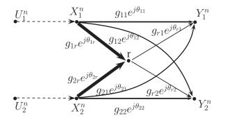
Figure 3.3: Correlated sources and phase incoherent interference relay channel (PI-IRC).
