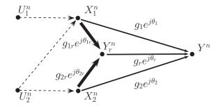
Figure 3.2: Correlated sources and phase incoherent non-causal cognitive multiple access relay channel (PI-NC-MARC). Moreover, (3.40)-(3.41) also describes sufficient conditions for reliable communications with
