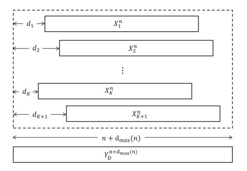
Figure 4.1: Gaussian time asynchronous multiple access relay channel (TA-MARC), with delays  $d_1, \dots, d_{K+1}$ .
