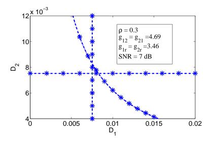
Figure 3.6: An achievable distortion region with  $\rho = 0.3$ ,  $P_1 = P_2 = P_r = 5$ , N = 1. All channel gains (except for  $g_{12}$ ,  $g_{21}$ ,  $g_{1r}$ ,  $g_{2r}$ ) are 1. The exact inner bound is sketched with starred lines whereas dashed lines depict the approximate inner bound.
