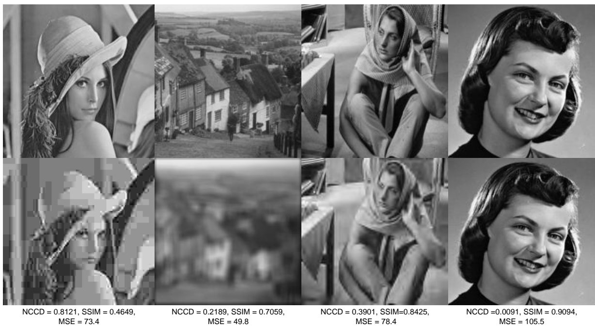
Figure 3.1: Comparison of MSE, SSIM and NCCD measures using images distorted by JPEG compression, blur, JPEG2000 compression and contrast reduction.
