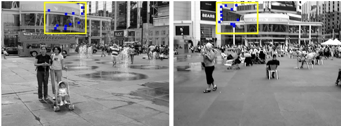
Figure 3.4: Feature extraction for frame matching. Both images have been divided to M sub-frames with minimum N features. Hamming Distance is used to find the best match between frames of local video and taken users' shot.
