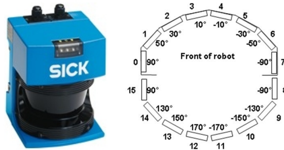
(a) SICK LMS [11]. (b) Lower Sonar Array [47].
