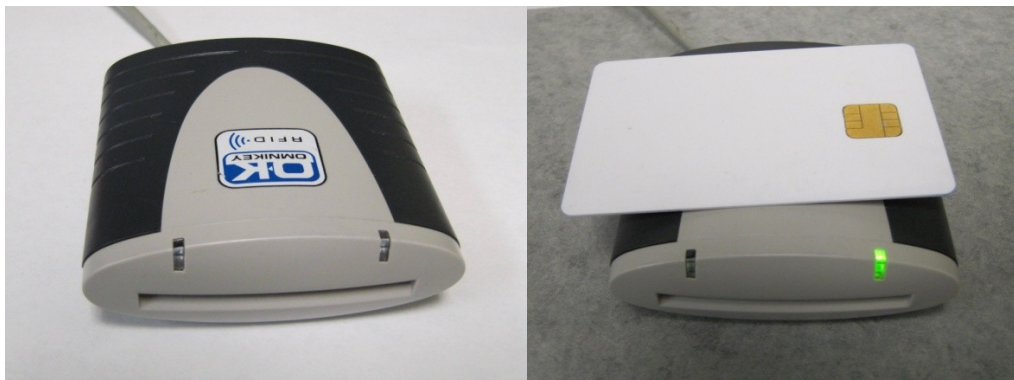
Figure 6.1: CardMan 5121, dual interface card reader
