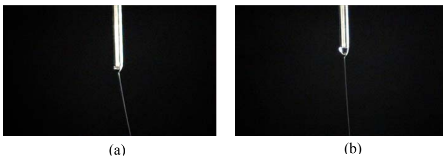
Fig. 7.6: Behaviour of the electrospun jet from a glycerol droplet with the application of high voltage to the needle electrode: (a) positive and (b) negative.
