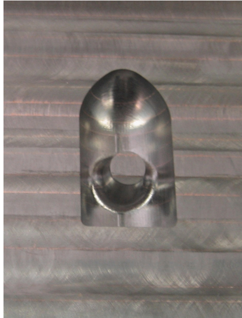
Figure 6-5: Inside of the cavity and joined layers
