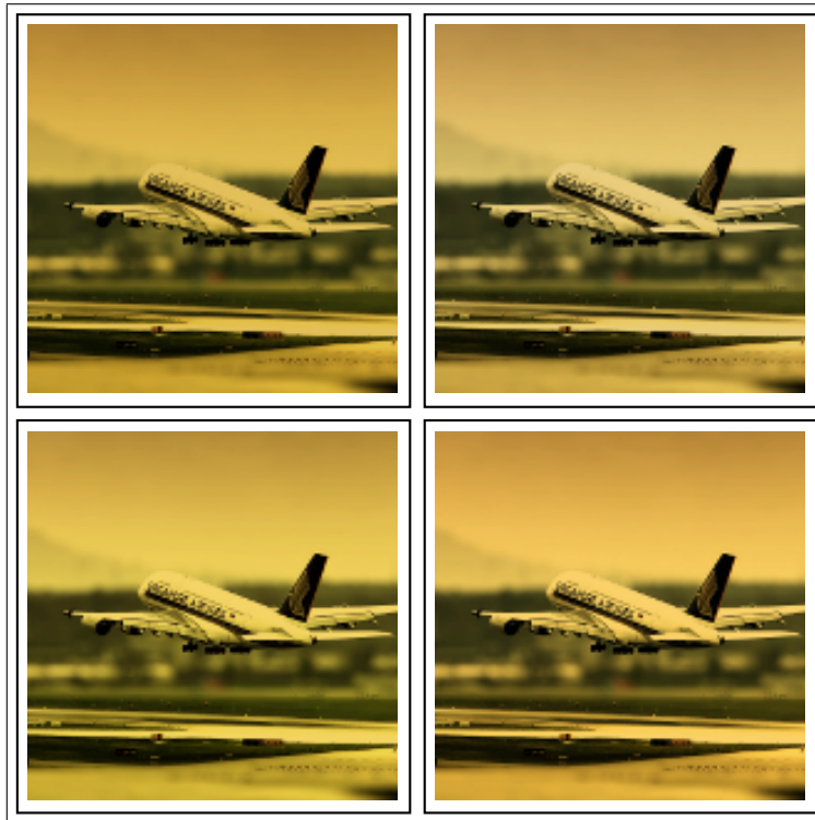
Figure 5.14: Adjusted images for displaying under illuminant A. Top left: CIECAM02. Top right: Fairchild's. Bottom left: CIELAB. Bottom right: von Kries.
