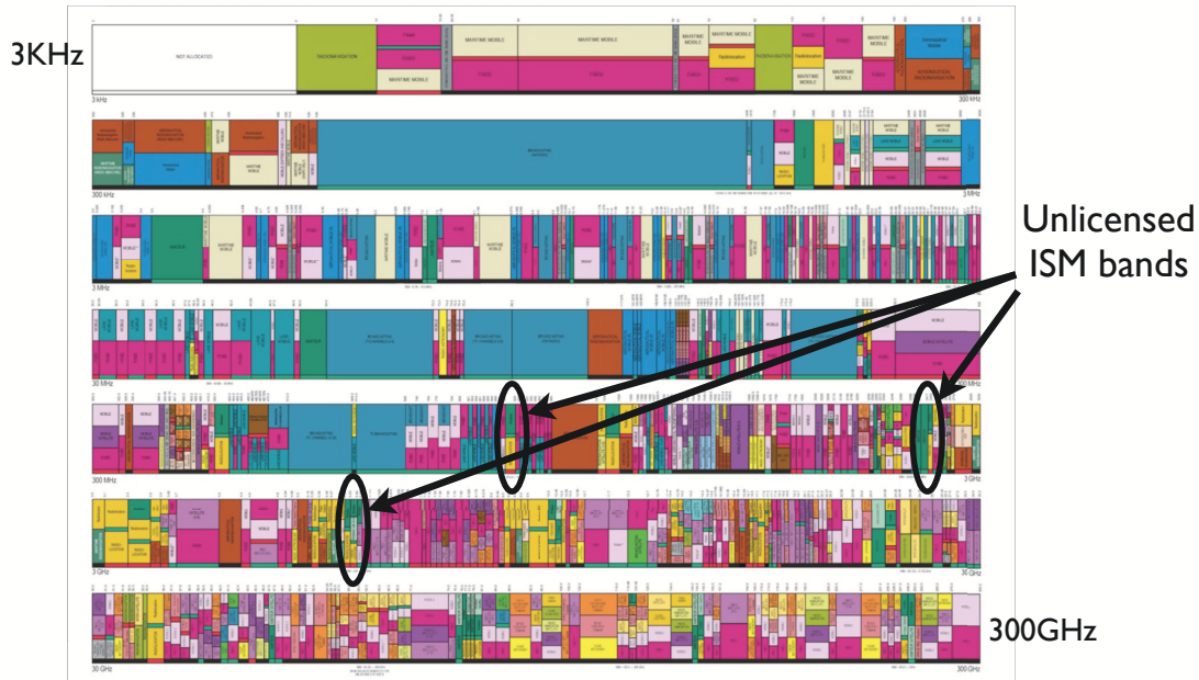
Figure 1.1: Allocation of RF Spectrum by the Federal Communications Commission (FCC) in the US
