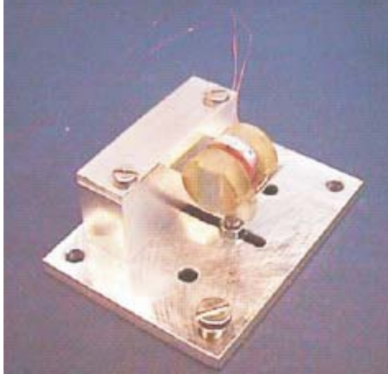
Figure 2.7: Improved electromagnetic MPG described in [49].
