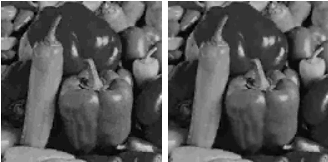
Fig 6.3 Reconstructed images (multiplierless version with optimized 2-point prediction) at CR=114.51, (left) before postprocessing PSNR=27.73dB, and (right) after postprocessing PSNR=27.75dB.
