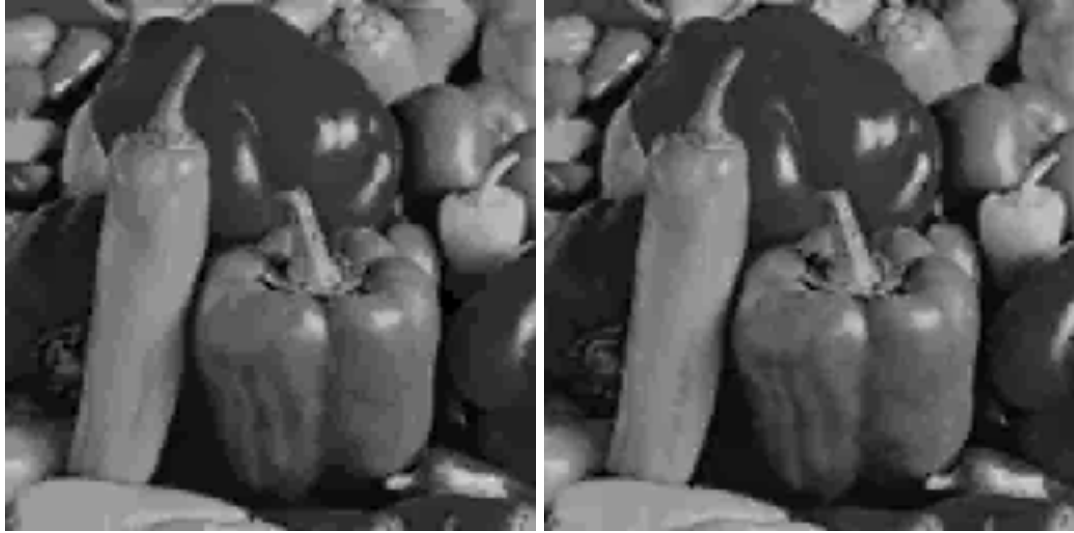
Fig 6.2 Reconstructed images, (left) 4-point prediction without optimization at CR=103.0 and 27.45dB, and (right) 2-point prediction with optimization at CR=105.5 and 27.9dB.
