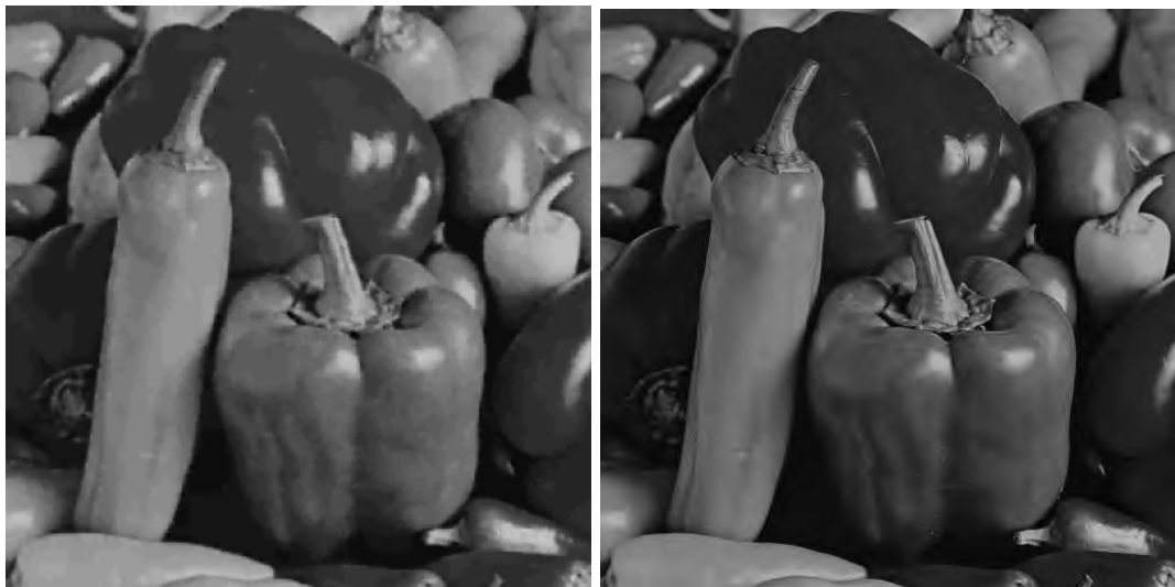
Fig 6.5 Reconstructed Images, (left) proposed at 35:1 and 31.1dB and (right) JPEG2000 at 33:1 and 22.7dB.
