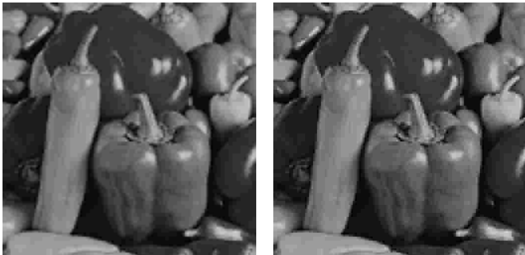
Fig 4.3 Reconstructed images at 62:1 compression using 8x8 blocks (left) with boundary interpolation at 28.8dB and (right) no interpolation at 28.2dB.
