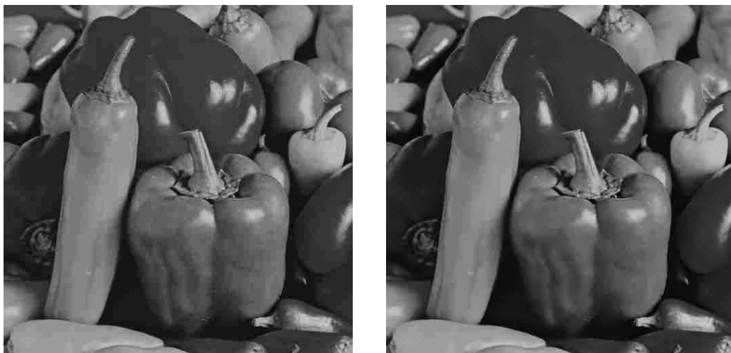
Fig 7.3 Reconstructed JPEG images (left) before postprocessing PSNR=32.2dB and (right) after postprocessing PSNR=32.4dB
