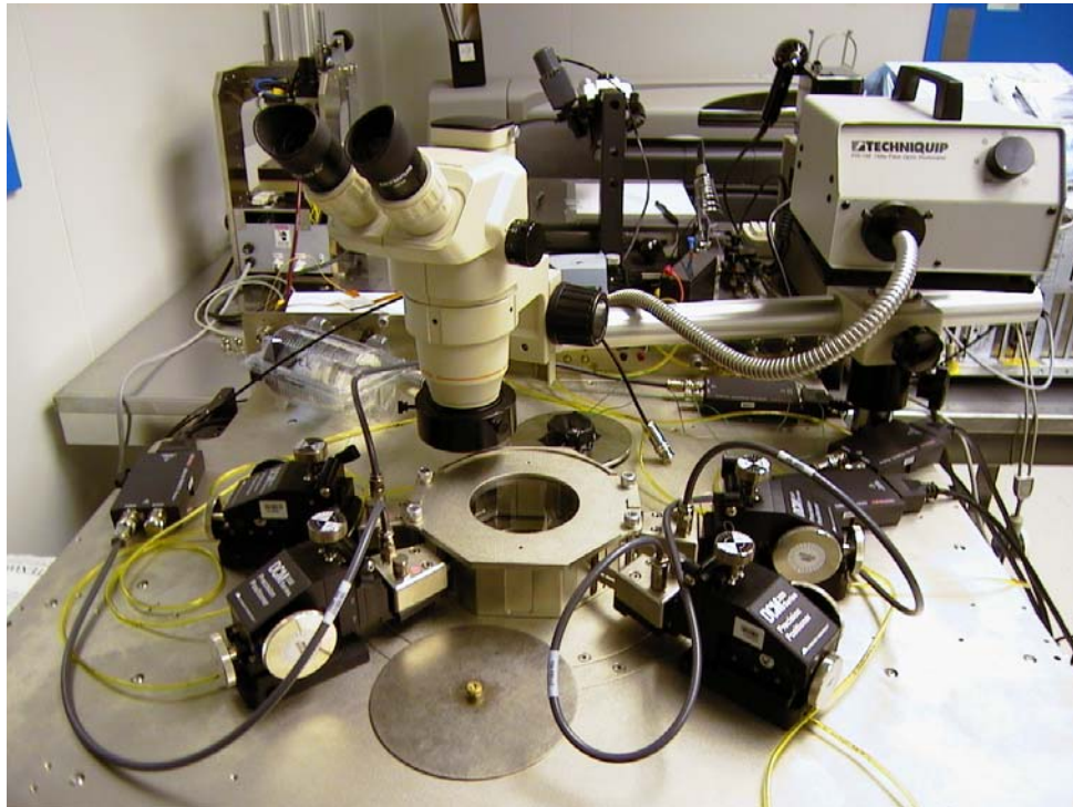
Figure 5-12: Cascade low noise prober for wafer testing.
