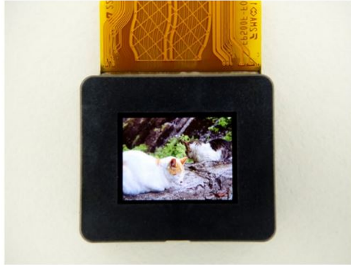
Figure 1.2: Photograph of the output image by 0.5-inch UXGA OLED microdisplay [2].
