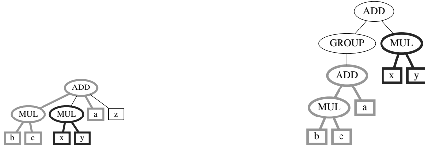
Figure 3.2: Matching multiple formula subtrees between the OPT representations of formulas a+bc+xy+z and (a+bc)+xy as shown in the left and right of the figure respectively.
