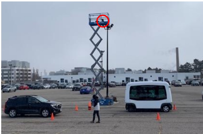
Figure 5.3: Intersection scenario with WATonoBus, another vehicle, and a pedestrian
