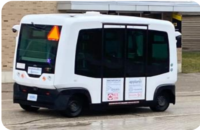
Figure 5.2: WATonoBus, an autonomous shuttle bus with Vehicle to Infrastructure (V2I) connectivity
