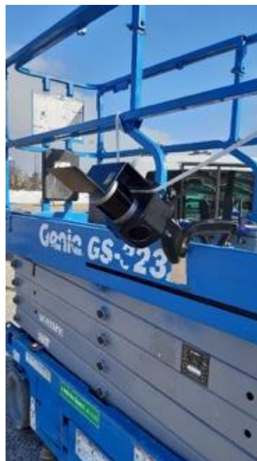
Figure 5.1: ISN, including two cameras and a Lidar, mounted on a scissor lift
