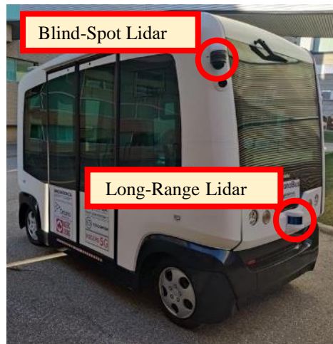
Figure 5.2: The WATonoBus platform is used for experimental studies of the developed self-localization system. The vehicle is equipped with a long-range 32-beam Lidar with a vertical Field of View (FOV) of 40^\circ and horizontal FOV of 180^\circ with up to 200 m range and \pm 3 cm accuracy. A short-range 32-beam blind spot Lidar is used with 360^\circ horizontal FOV, 90^\circ vertical FOV, and a range of 30m with up to \pm 3 cm typical range accuracy. The short-range Lidar is used for scanning nearby curbs. The long-range Lidar scans building planes and poles. The vehicle is equipped with an RTK-GNSS-INS with centimeter-level accuracy that provides the ground truth information of the self-localization.
