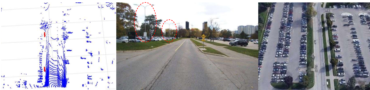
Figure 5.15: The environment contains mostly temporarily parked vehicles while lacking enough longitudinal and lateral excitation. HD-LOC solely attends to the light poles (denoted in red) to localize the vehicle while filtering out the rest of the point cloud.
