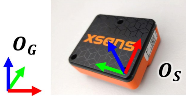
Figure 6-4 Global frame \mathbf{O}_G and sensor frame \mathbf{O}_S defined by an IMU.
