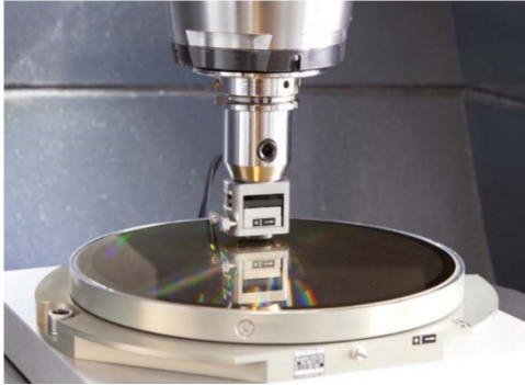
Figure 2-34 Grid encoder (KGM) [89].
